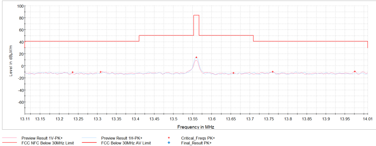
Plot 7-7. In Band Radiated Spurious Emissions (Reader A 848kbps, AC/DC Adapter and Magnetic Charger)
