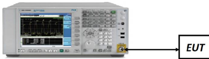
Figure 7-6. Test Instrument & Measurement Setup
