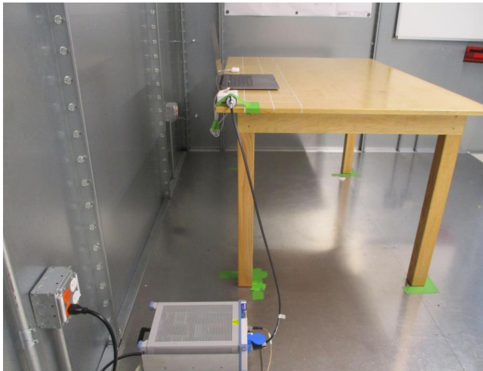
Figure 4: AC Line Conducted Emissions (Side View)
