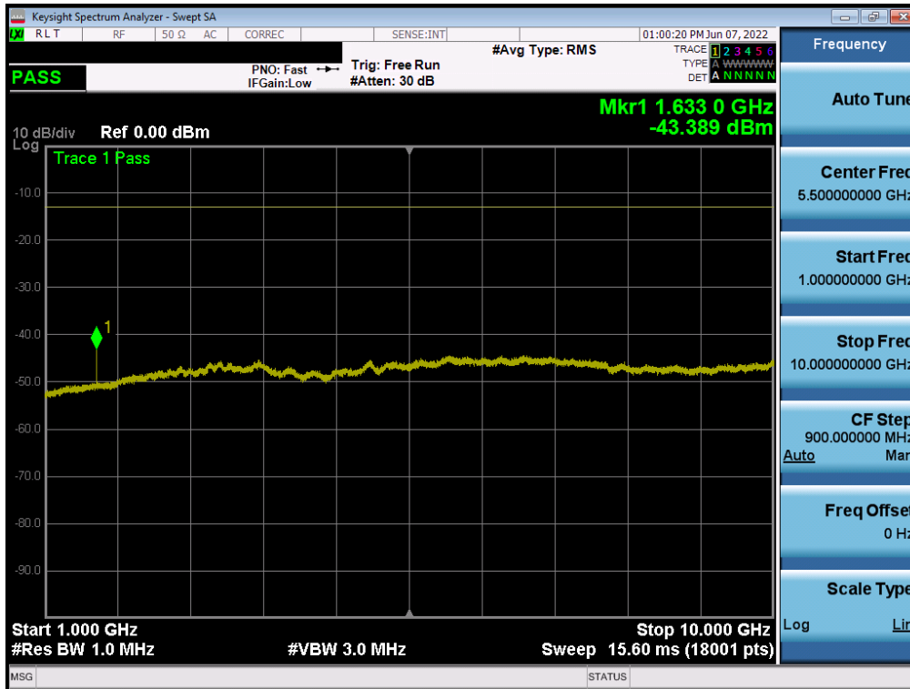
Plot 7-15. Conducted Spurious Plot (LTE Band 26 - 5MHz QPSK - RB Size 1, RB Offset 0 – Low Channel)
