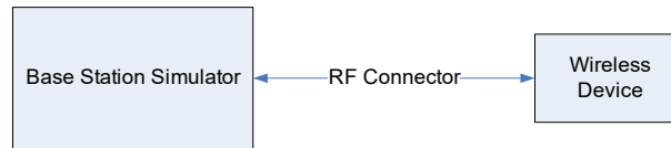
Figure 8-2 Power Measurement Setup
