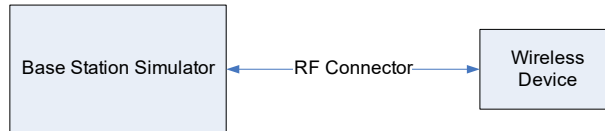
Figure 8-1 Power Measurement Setup
