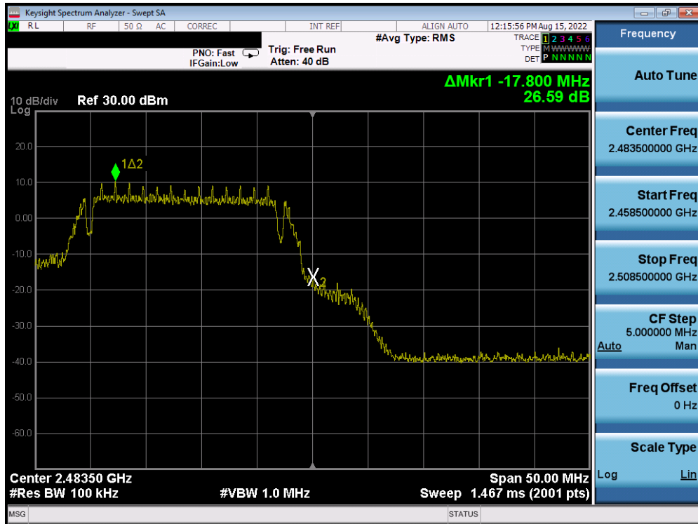
Plot 7-36. Band Edge Plot (802.11g – Ch. 13) – 6Mbps
