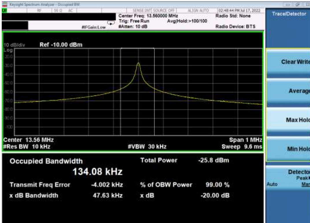
Plot 7-2. 20dB and 99% Bandwidth Plot (CE B 106kbps)
