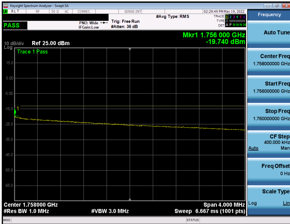
Plot 7-95. Upper Extended Band Edge Plot (LTE Band 4 - 10MHz QPSK – Full RB)
