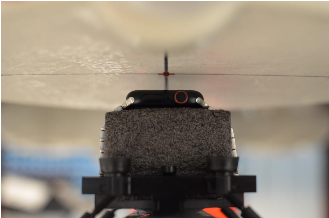
SAR Test Setup Photo 2: Aluminum with Metal Links Wristband, Head, Front Side at 10 mm
