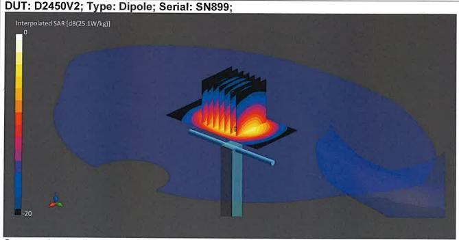
Communication System: CW UID: 0; Frequency: 2450.0 MHz; Duty Cycle: 1;
