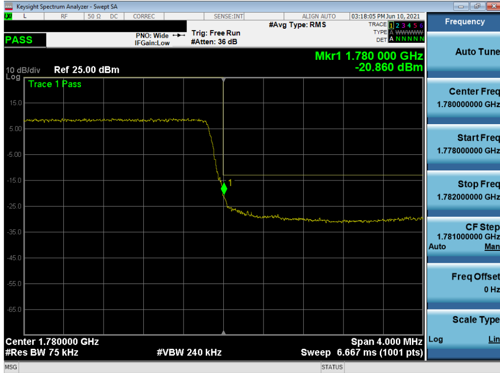
Plot 7-38. Upper Band Edge Plot (LTE Band 66 - 3MHz QPSK – Full RB)
