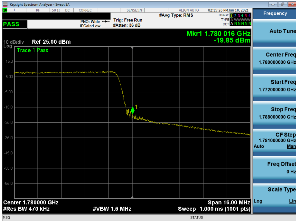
Plot 7-54. Upper Band Edge Plot (LTE Band 66 - 20MHz QPSK – Full RB)
