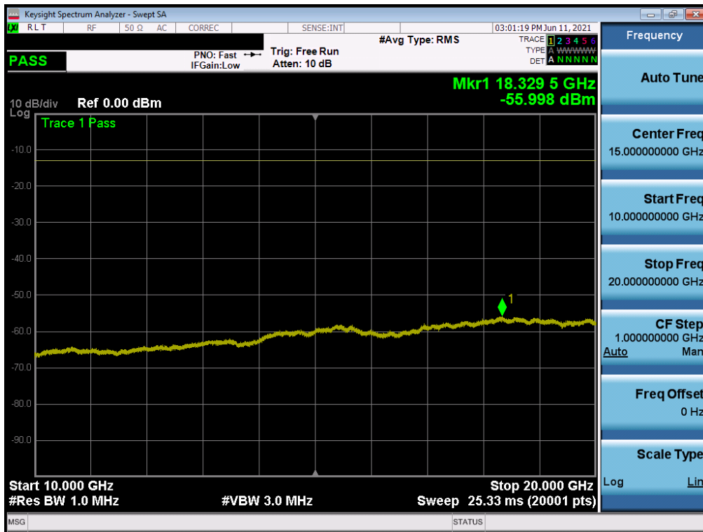
Plot 7-28. Conducted Spurious Plot (WCDMA Ch. 1413- Mid Channel)
