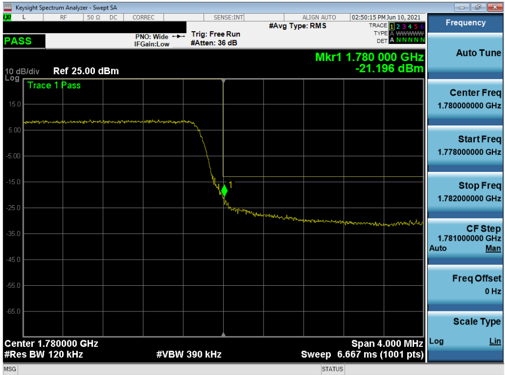
Plot 7-42. Upper Band Edge Plot (LTE Band 66 - 5MHz QPSK – Full RB)
