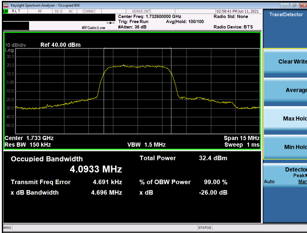
Plot 7-13. Occupied Bandwidth Plot (WCDMA, Ch. 1413)
