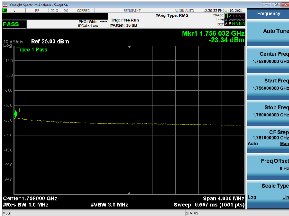
Plot 7-75. Upper Extended Band Edge Plot (LTE Band 4 - 15MHz QPSK – Full RB)
