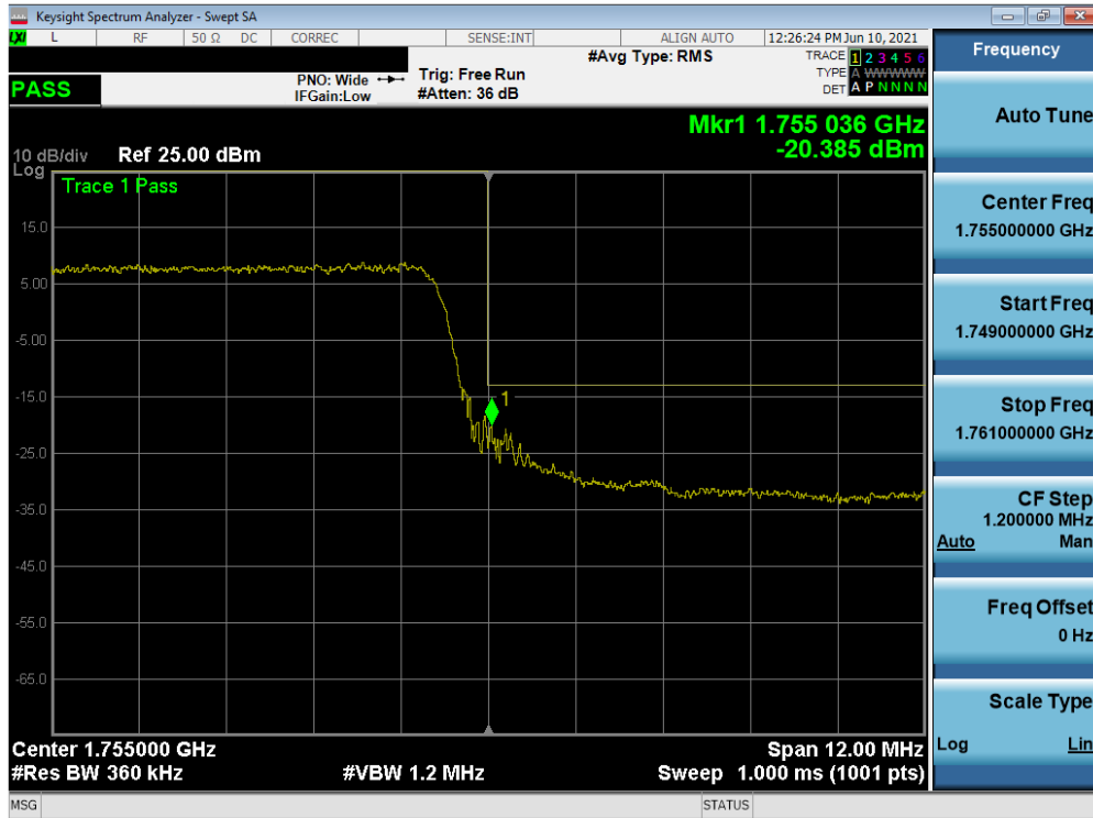
Plot 7-74. Upper Band Edge Plot (LTE Band 4 - 15MHz QPSK – Full RB)
