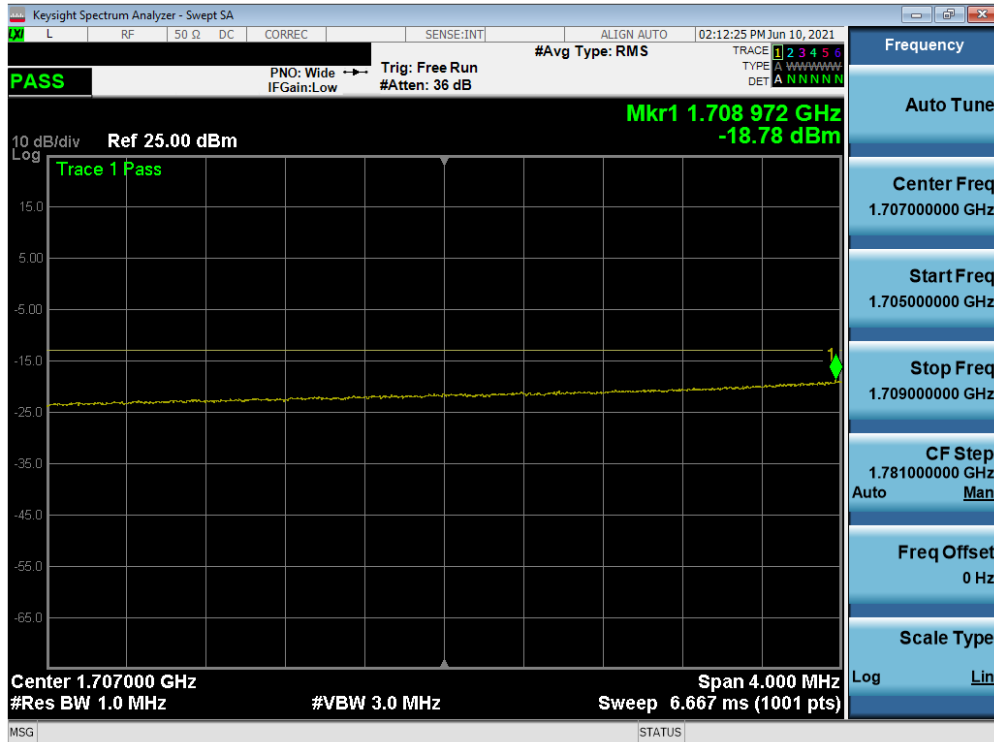
Plot 7-53. Lower Extended Band Edge Plot (LTE Band 66 - 20MHz QPSK – Full RB)
