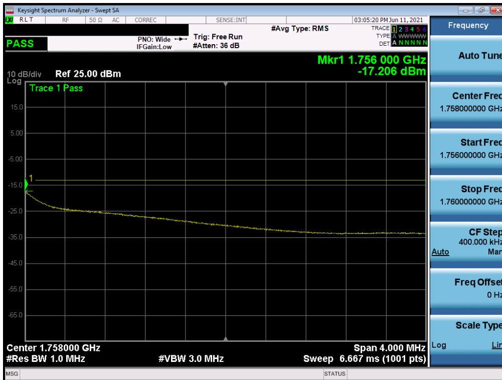
Plot 7-83. Upper Extended Band Edge Plot (WCDMA AWS – Ch. 1513)
