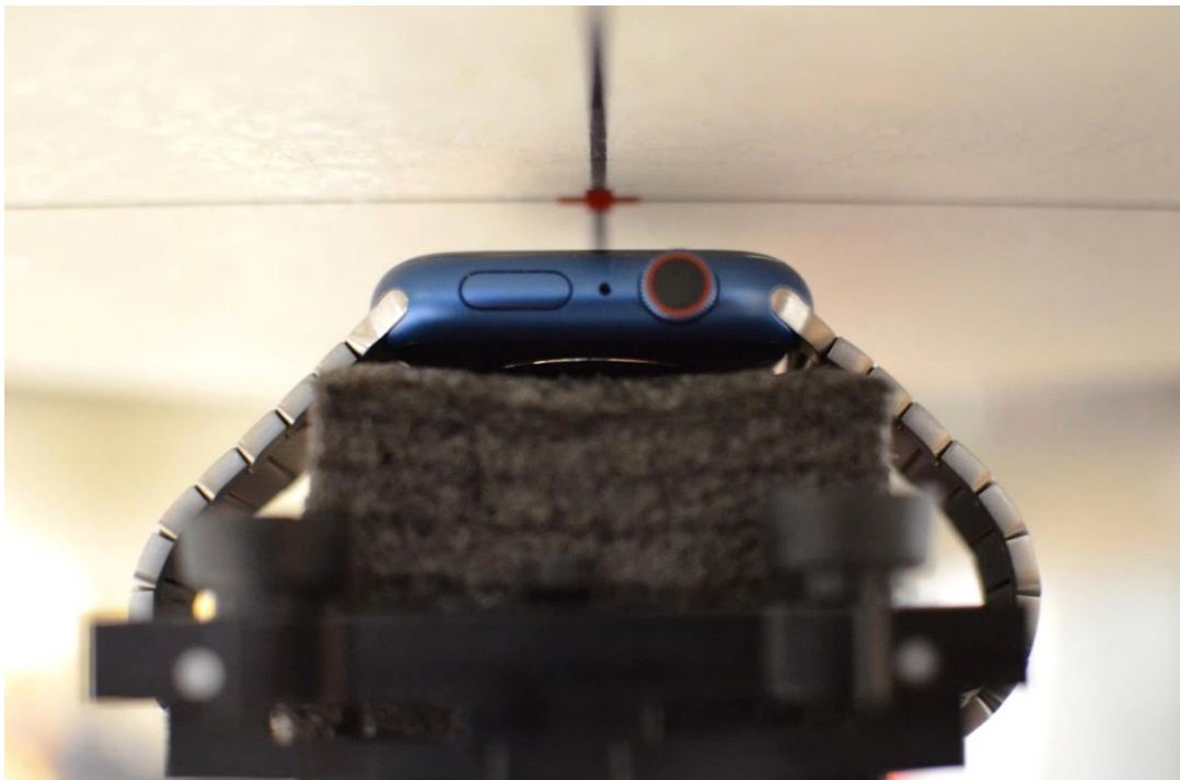
SAR Test Setup Photo 2 – Aluminum with Metal Links Wristband, Head, Front Side at 1.0 cm
