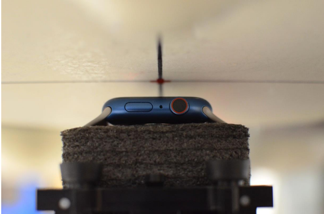
SAR Test Setup Photo 1 – Aluminum with Sport Wristband, Head, Front Side at 1.0 cm
