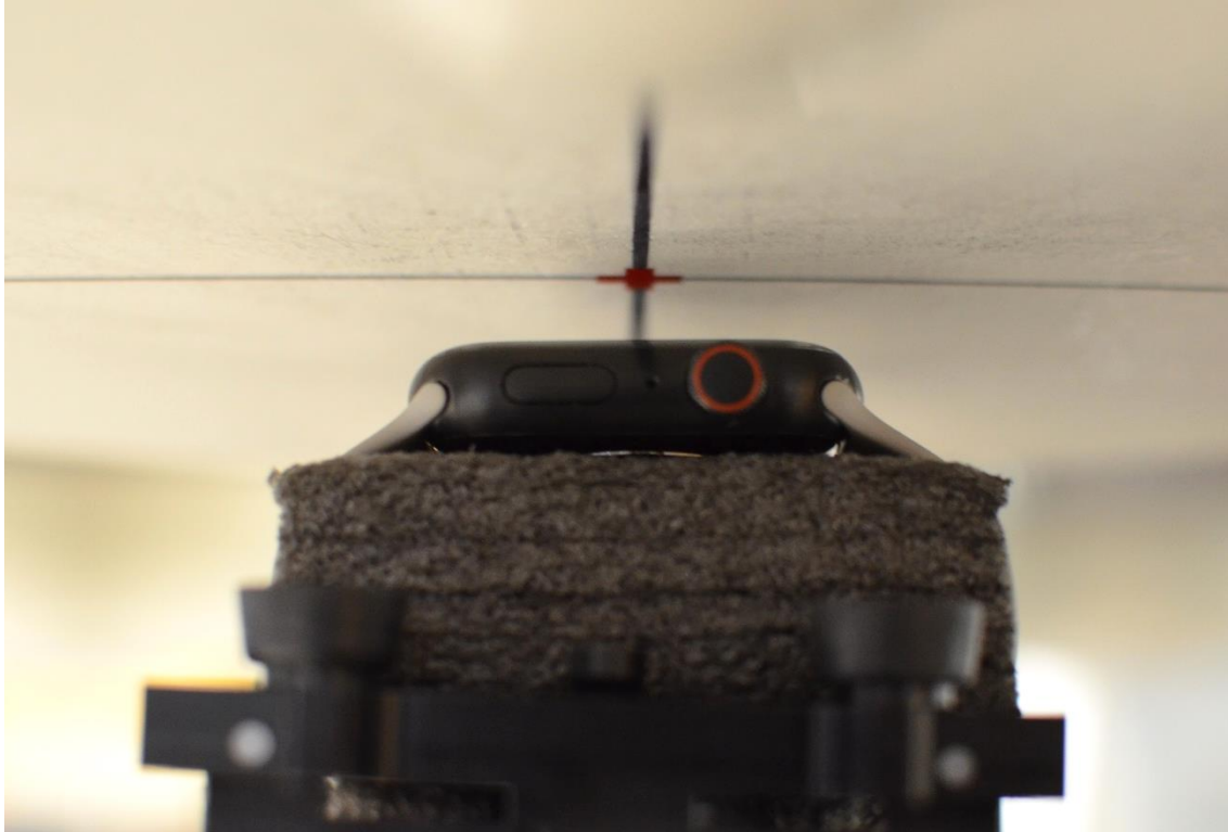
SAR Test Setup Photo 7 – Titanium with Sport Wristband, Head, Front Side at 1.0 cm
