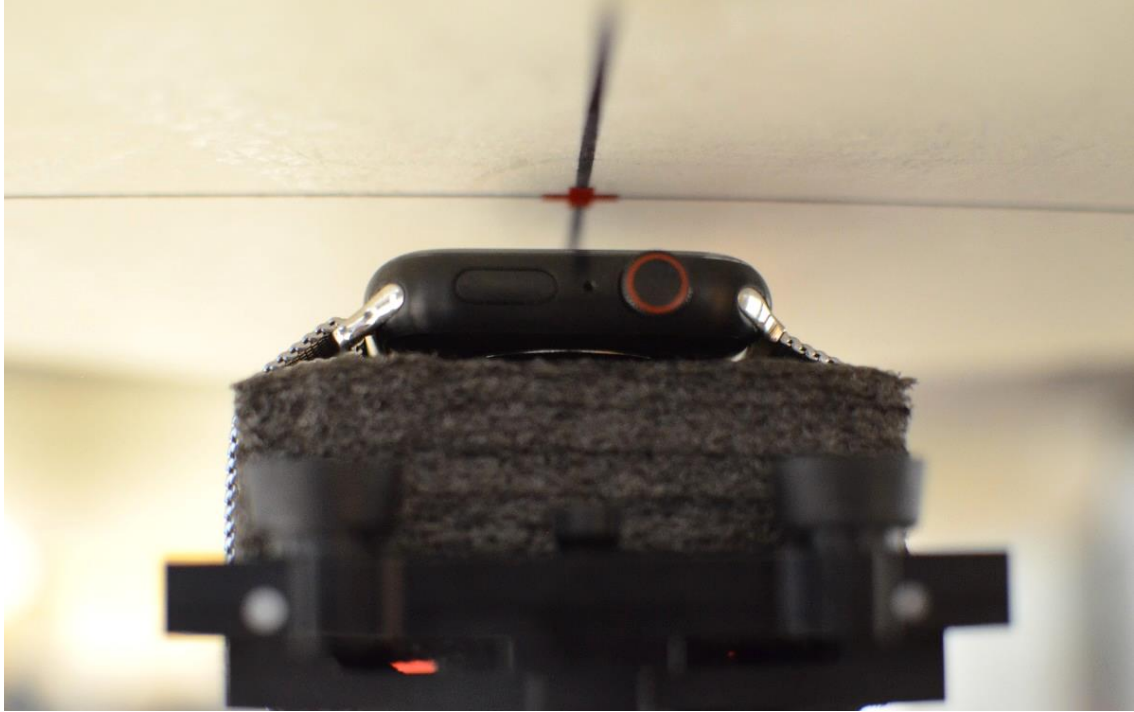
SAR Test Setup Photo 9 – Titanium with Metal Loop Wristband, Head, Front Side at 1.0 cm
