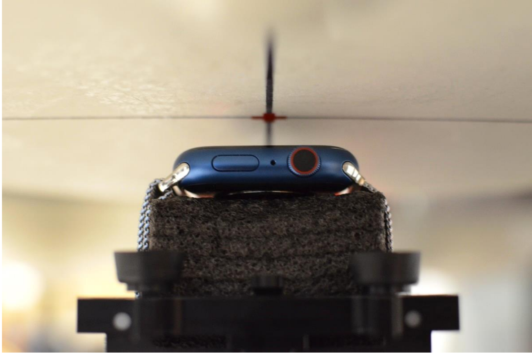
SAR Test Setup Photo 3 – Aluminum with Metal Loop Wristband, Head, Front Side at 1.0 cm
