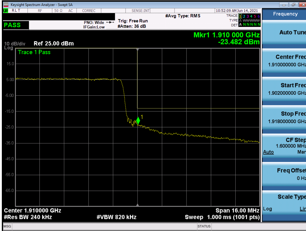
Plot 7-54. Upper Band Edge Plot (LTE Band 2 – 20MHz QPSK – Full RB Configuration)
