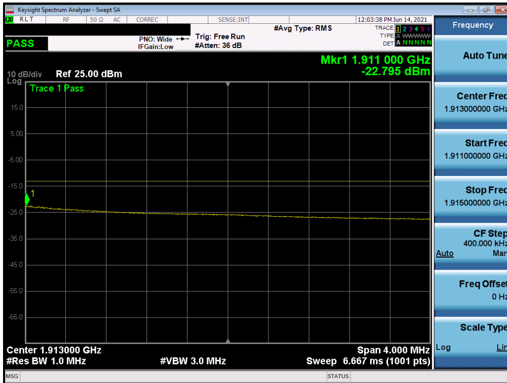
Plot 7-51. Extended Upper Band Edge Plot (LTE Band 2 – 15MHz QPSK – Full RB Configuration)
