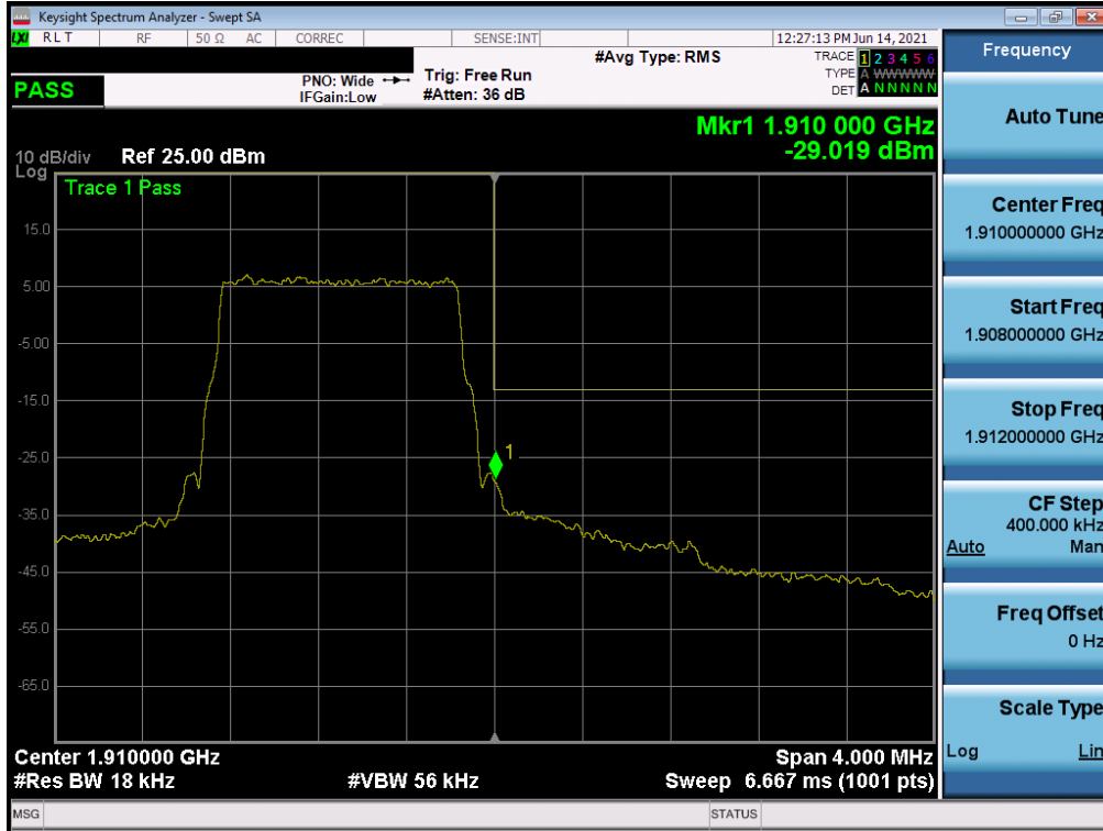
Plot 7-34. Upper Band Edge Plot (LTE Band 2 – 1.4MHz QPSK – Full RB Configuration)
