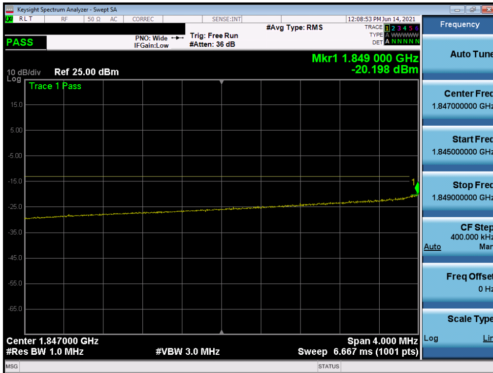
Plot 7-45. Extended Lower Band Edge Plot (LTE Band 2 – 10MHz QPSK – Full RB Configuration)
