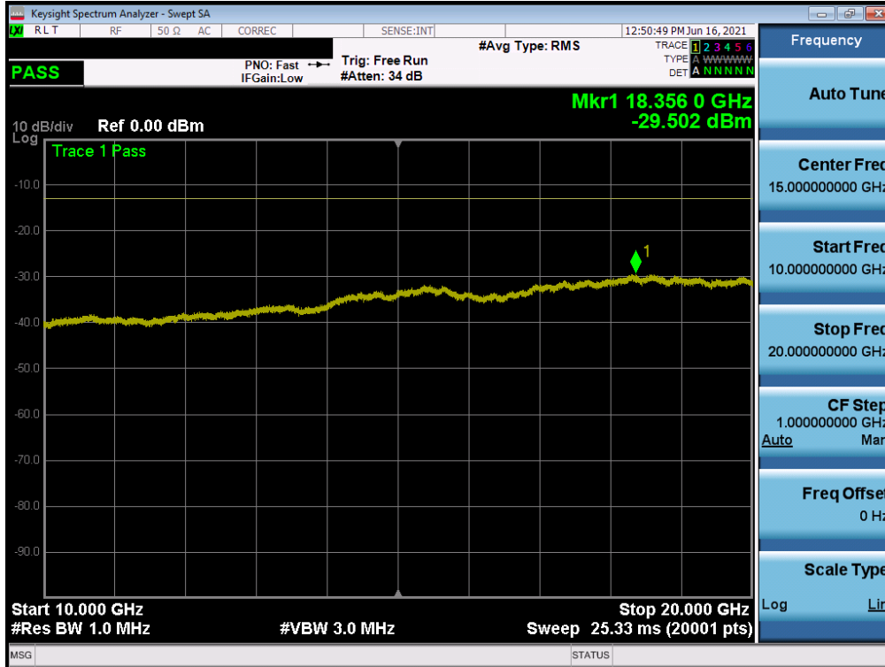
Plot 7-16. Conducted Spurious Plot (LTE Band 25/2 - 20MHz QPSK - RB Size 1, RB Offset 0 - Low Channel)
