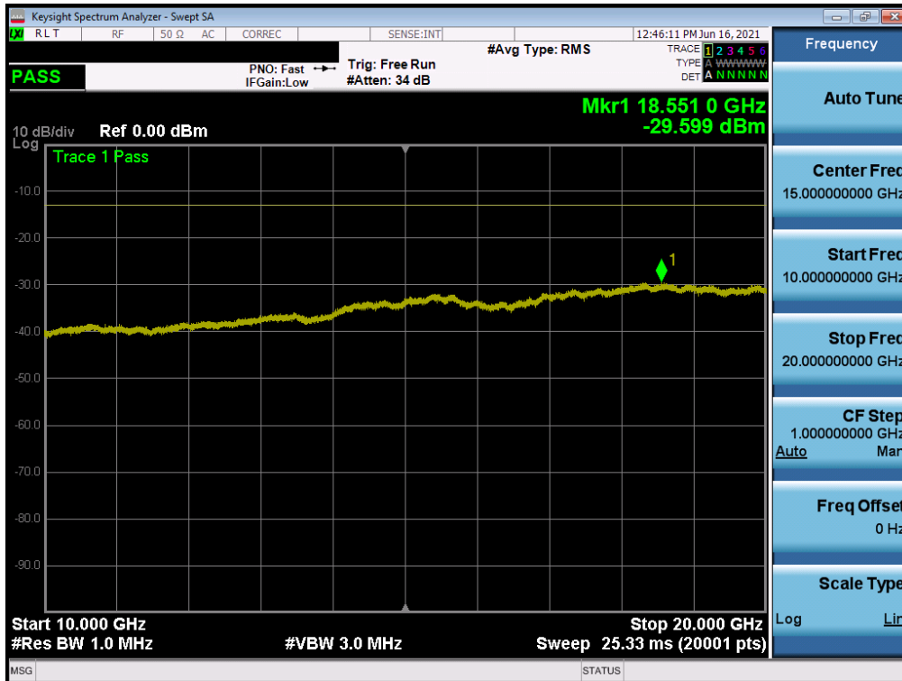
Plot 7-19. Conducted Spurious Plot (LTE Band 25/2 - 20MHz QPSK - RB Size 1, RB Offset 0 - Mid Channel)
