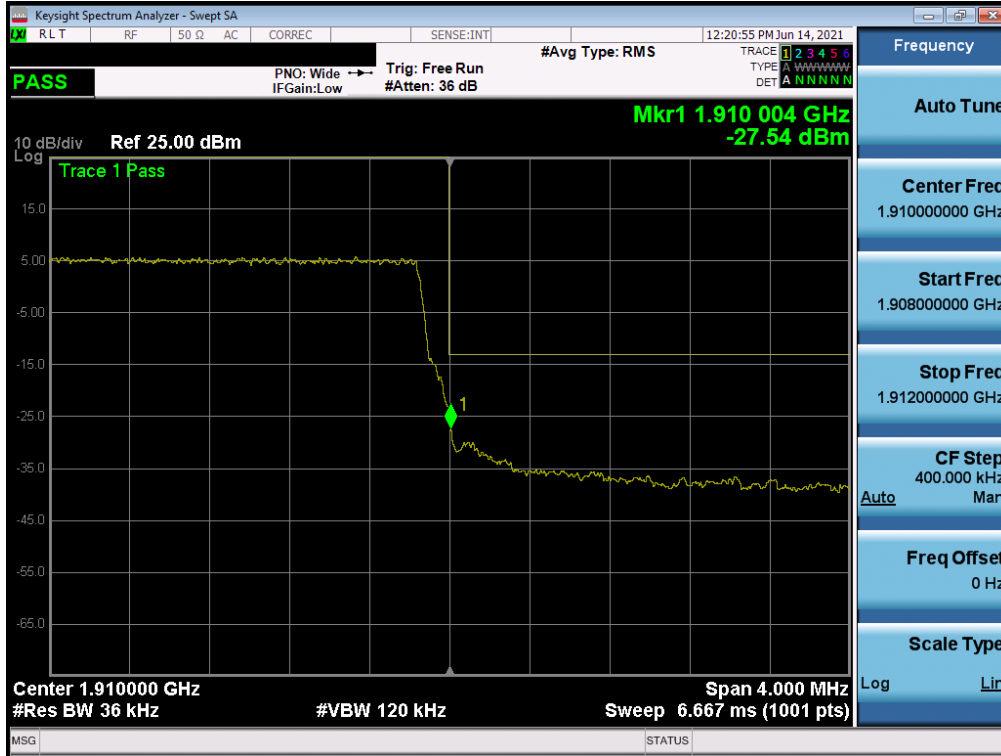
Plot 7-38. Upper Band Edge Plot (LTE Band 2 – 3MHz QPSK – Full RB Configuration)
