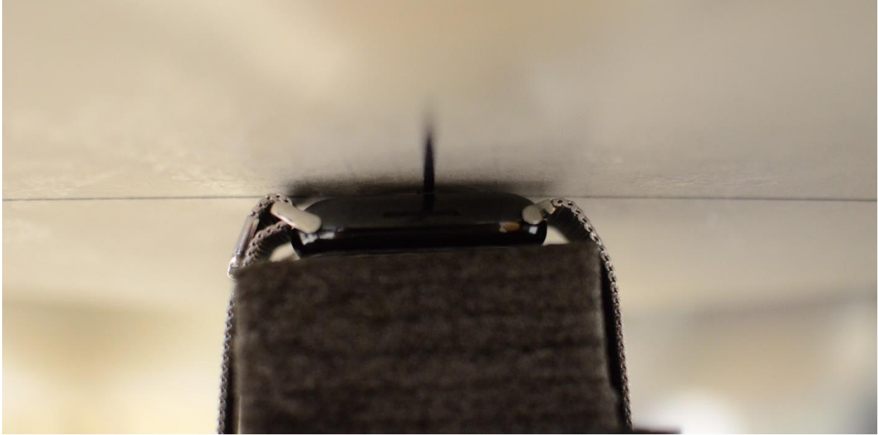
SAR Test Setup Photo 15: Stainless Steel with Metal Loop Wristband, Extremity, Back side at 0.0 cm
