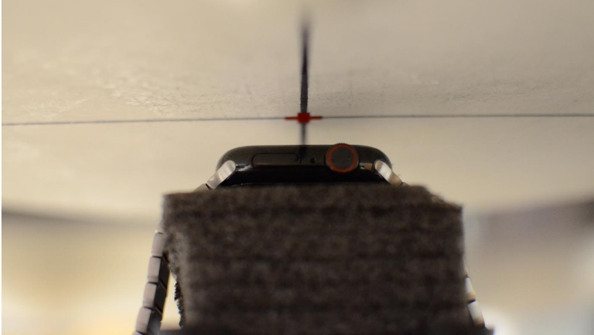
SAR Test Setup Photo 5: Stainless Steel with Metal Links Wristband, Head, Front side at 1.0 cm
