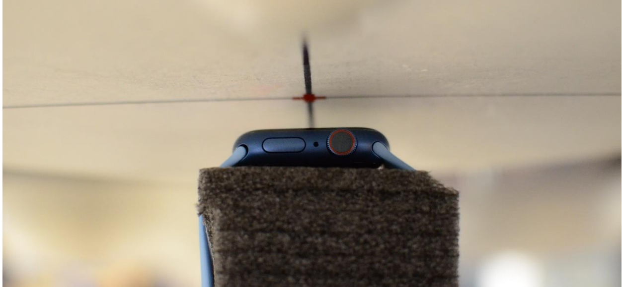
SAR Test Setup Photo 1: Aluminum with Sport Wristband, Head, Front side at 1.0 cm
