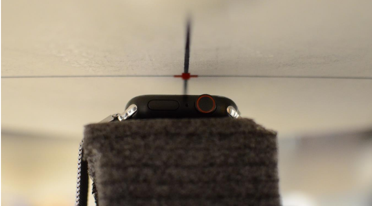
SAR Test Setup Photo 9: Titanium with Metal Loop Wristband, Head, Front side at 1.0 cm
