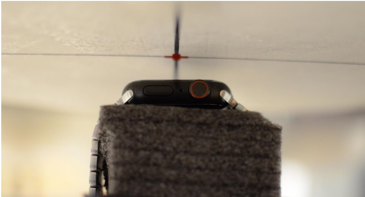
SAR Test Setup Photo 8: Titanium with Metal Links Wristband, Head, Front side at 1.0 cm
