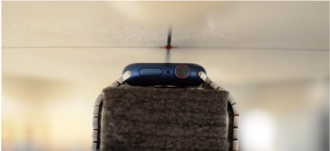
SAR Test Setup Photo 2: Aluminum with Metal Links Wristband, Head, Front side at 1.0 cm
