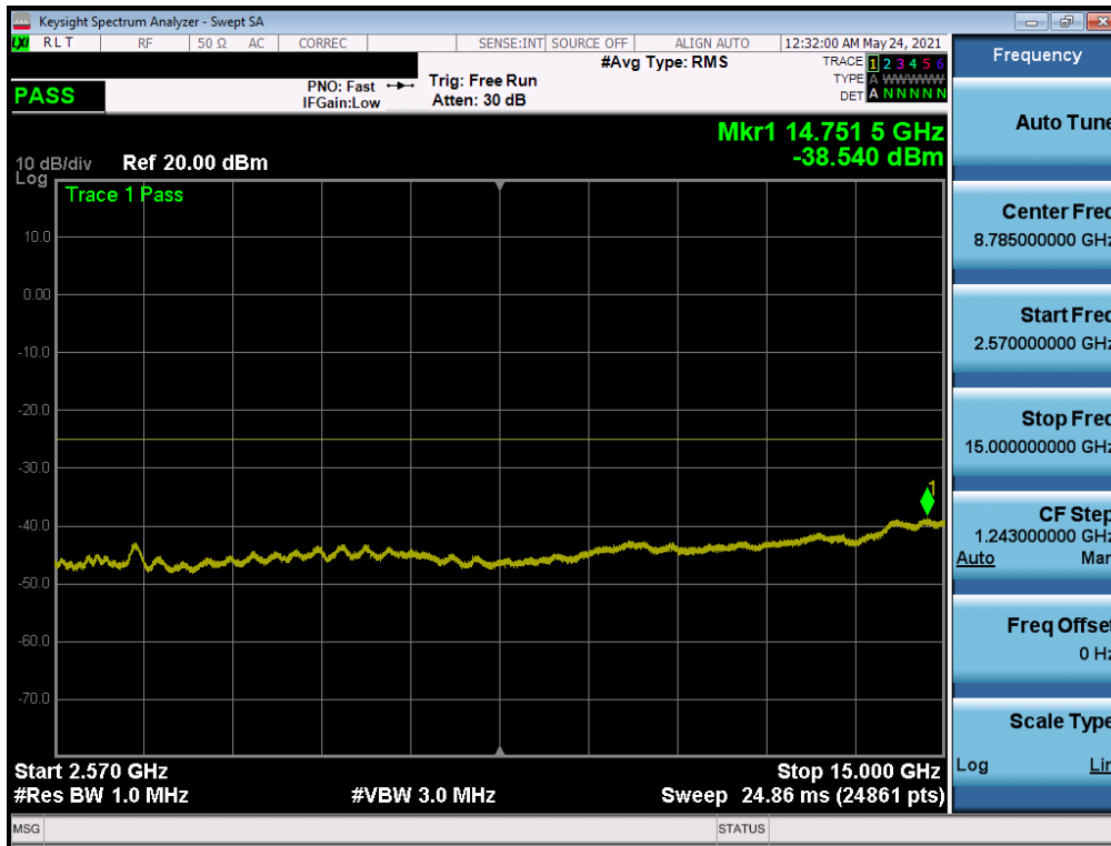
Plot 7-18. Conducted Spurious Plot (LTE Band 7 - 20MHz QPSK - RB Size 1, RB Offset 0 - Low Channel)
