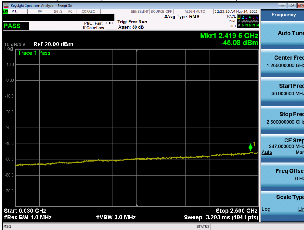
Plot 7-20. Conducted Spurious Plot (LTE Band 7 - 20MHz QPSK - RB Size 1, RB Offset 0 - Mid Channel)
