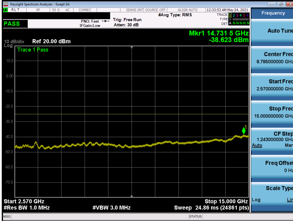
Plot 7-21. Conducted Spurious Plot (LTE Band 7 - 20MHz QPSK - RB Size 1, RB Offset 0 - Mid Channel)
