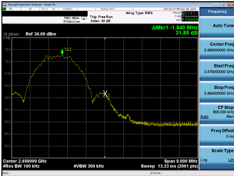
Plot 7-22. Band Edge Plot (Bluetooth (LE), 2Mbps, ePA – Ch. 38)
