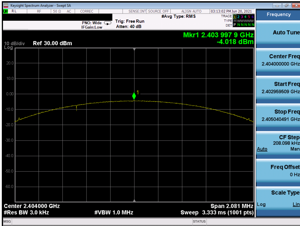
Plot 7-13. Power Spectral Density Plot (Bluetooth (LE), 2Mbps, ePA – Ch. 1)
