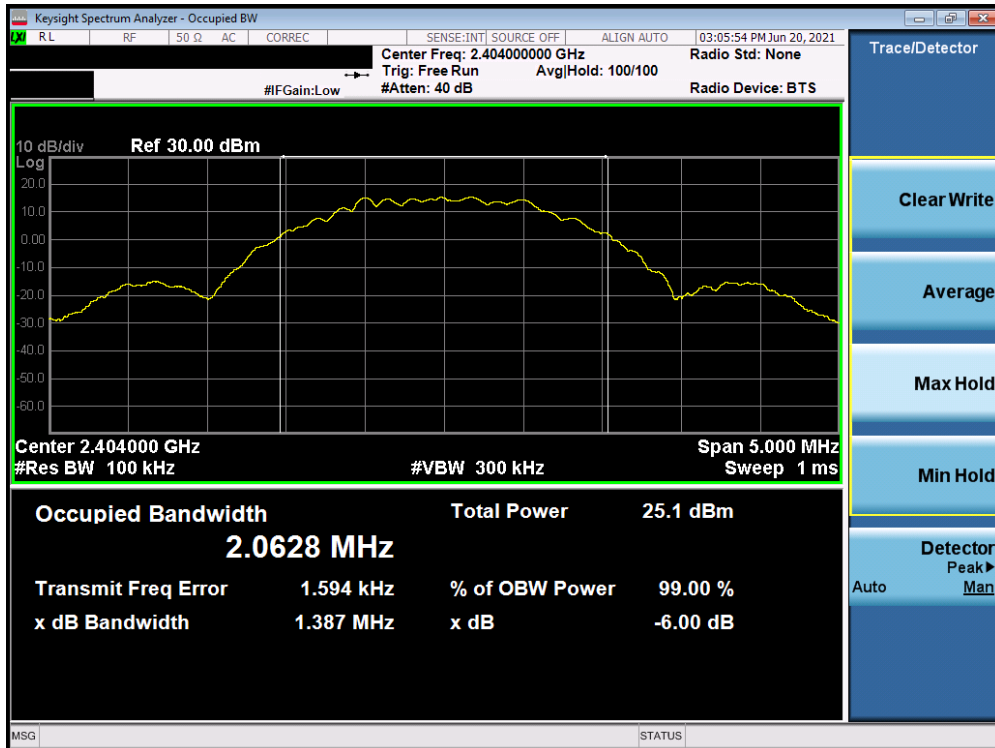
Plot 7-4. 6dB Bandwidth & 99% OBW Plot (Bluetooth (LE), 2Mbps, ePA – Ch.1)
