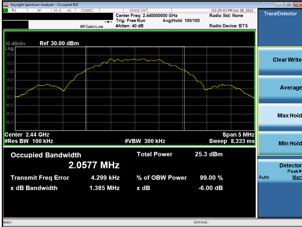
Plot 7-5. 6dB Bandwidth & 99% OBW Plot (Bluetooth (LE), 2Mbps, ePA – Ch. 19)
