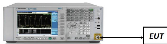
Figure 7-4. Test Instrument & Measurement Setup
