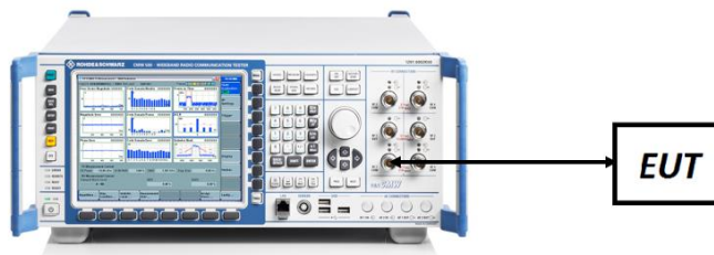
Figure 7-5. ERP/EIRP Measurement Setup
