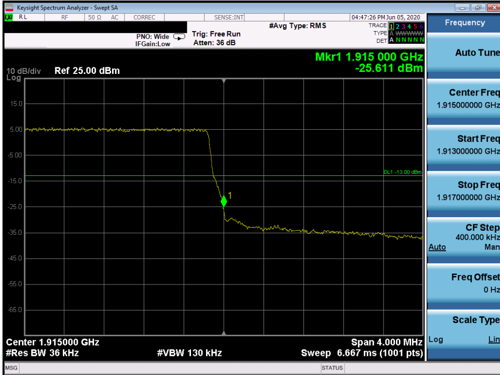
Plot 7-164. Upper Band Edge Plot (Band 25 - 3.0MHz QPSK - Full RB Configuration)
