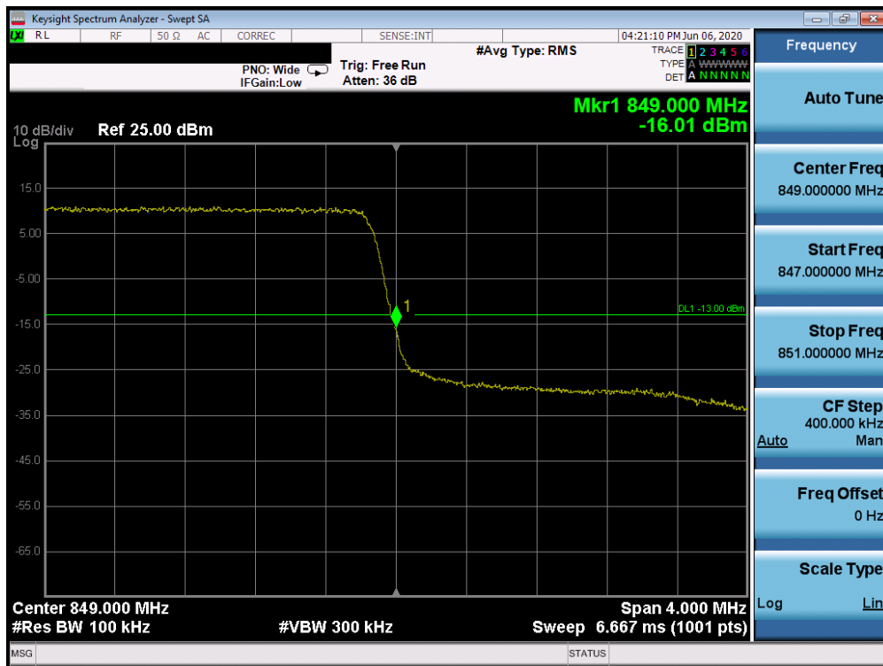
Plot 7-105. Upper Band Edge Plot (Band 5 - 3.0MHz QPSK - Full RB Configuration)
