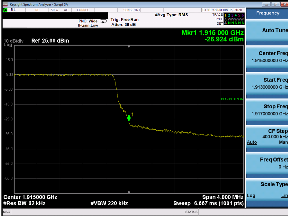
Plot 7-168. Upper Band Edge Plot (Band 25 - 5.0MHz QPSK - Full RB Configuration)
