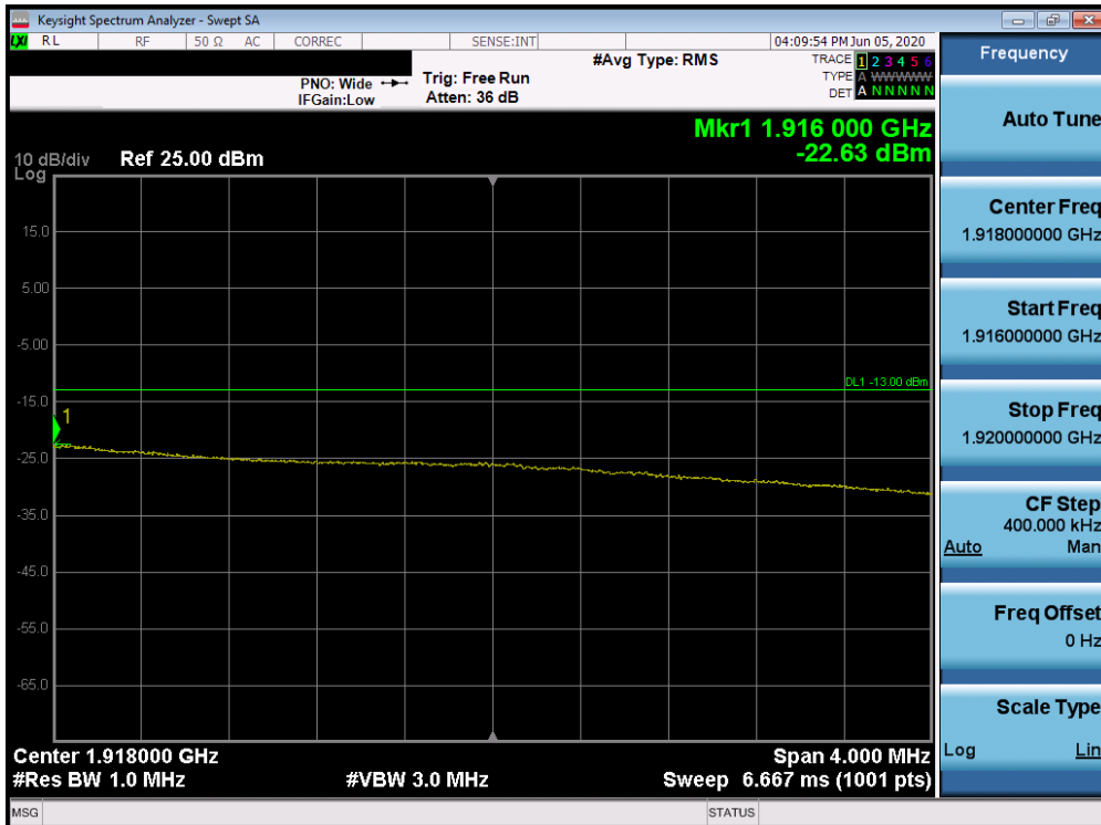
Plot 7-177. Upper Extended Band Edge Plot (Band 25 - 15.0MHz QPSK - Full RB Configuration)
