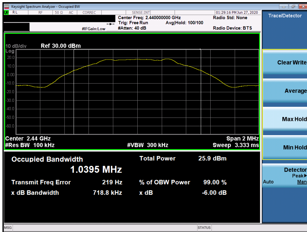
Plot 7-2. 6dB Bandwidth Plot (Bluetooth (LE), 1Mbps, ePA – Ch. 19)
