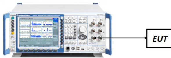
Figure 7-5. ERP/EIRP Measurement Setup
