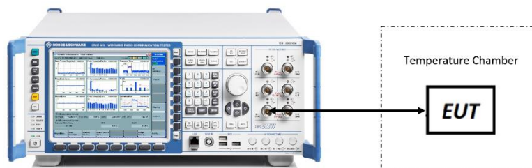
Figure 7-8. Test Instrument & Measurement Setup
