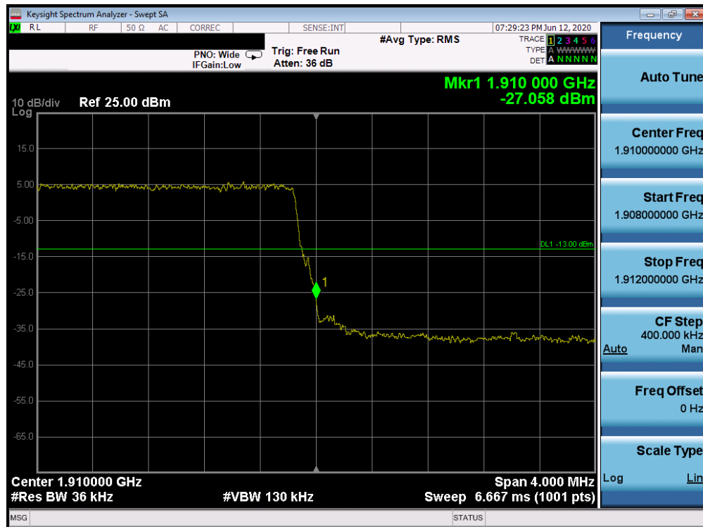
Plot 7-188. Upper Band Edge Plot (Band 2 - 3.0MHz QPSK - Full RB Configuration)
