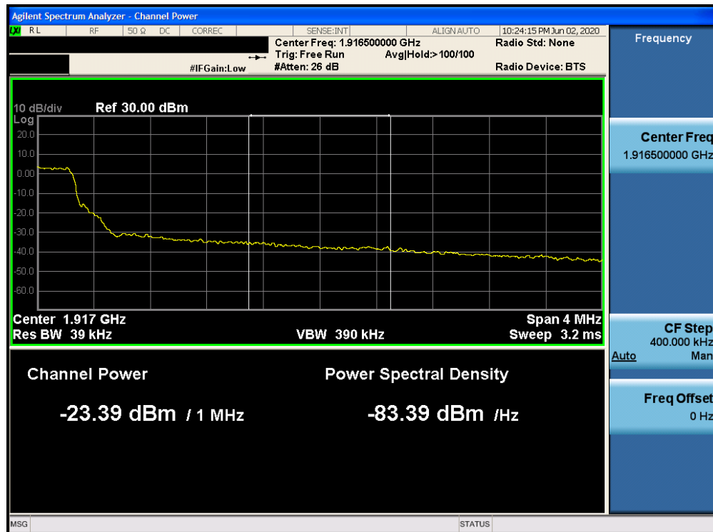
Plot 7-169. Upper Extended Band Edge Plot (Band 25 - 5.0MHz QPSK - Full RB Configuration)
