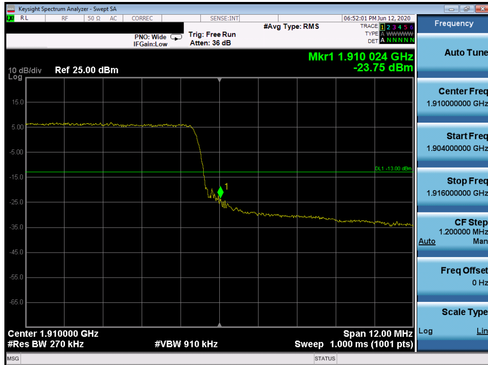
Plot 7-200. Upper Band Edge Plot (Band 2 - 15.0MHz QPSK - Full RB Configuration)
