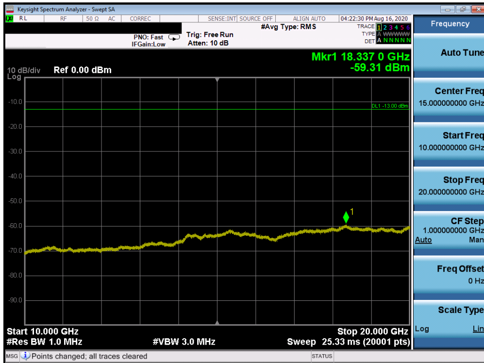
Plot 7-69. Conducted Spurious Plot (Band 25/2 - 20.0MHz QPSK - RB Size 1, RB Offset 0 - Low Channel)
