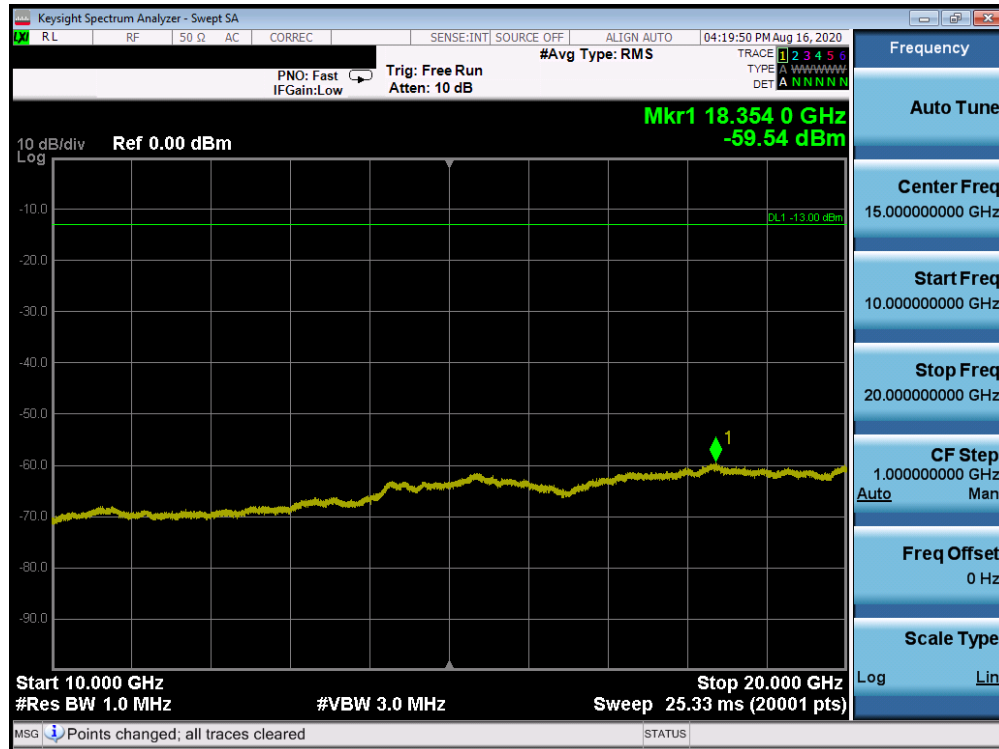
Plot 7-75. Conducted Spurious Plot (Band 25/2 - 20.0MHz QPSK - RB Size 1, RB Offset 0 - High Channel)
