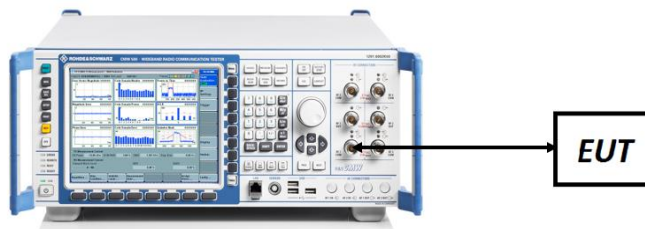
Figure 7-5. ERP/EIRP Measurement Setup
