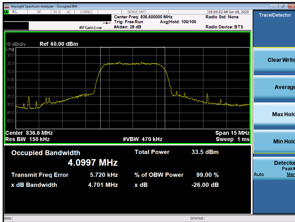
Plot 7-1. Occupied Bandwidth Plot (Cellular WCDMA Mode)
