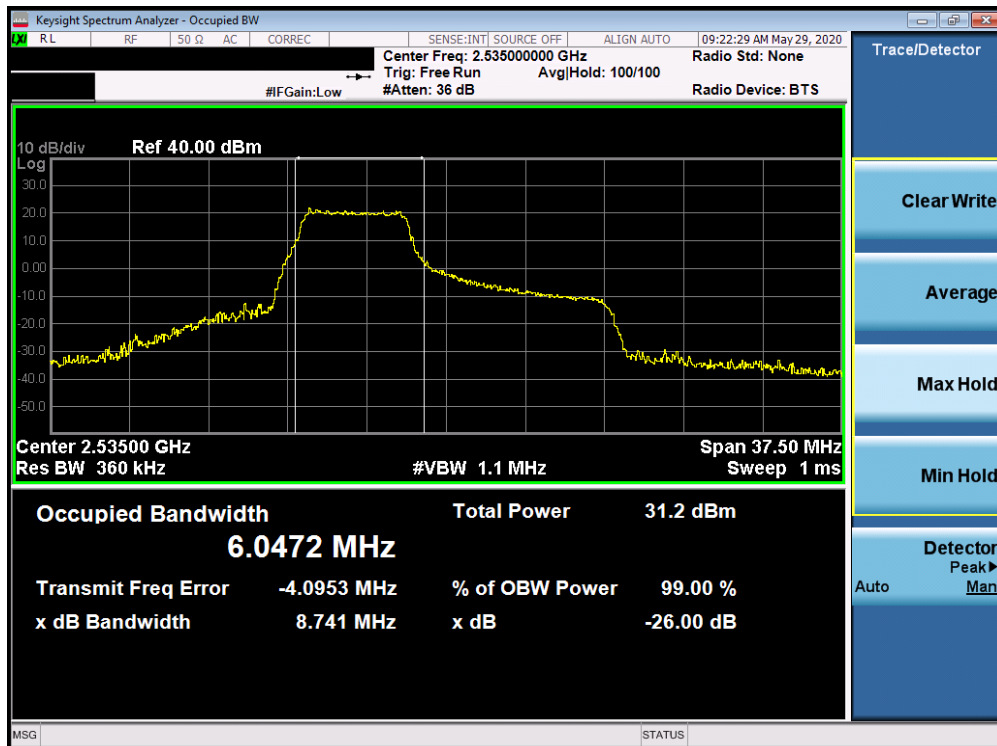
Plot 7-38. Occupied Bandwidth Plot (Band 7 - 15.0MHz 16-QAM - Full RB Configuration)
