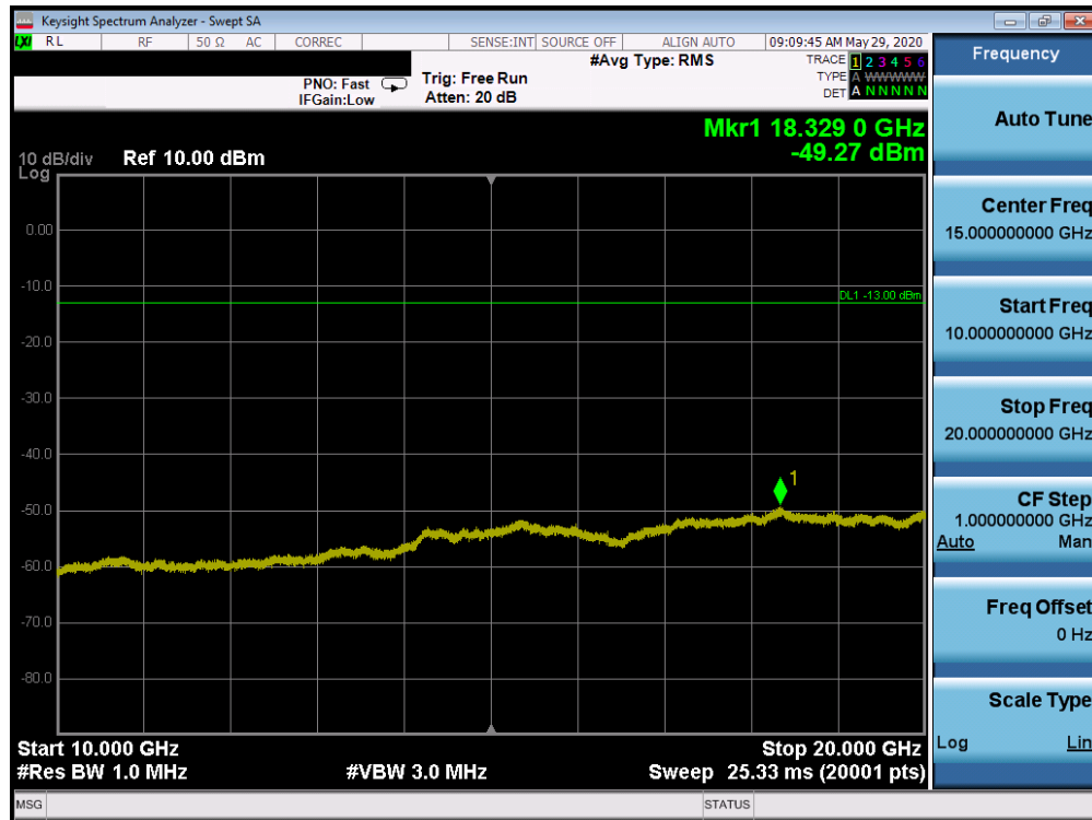
Plot 7-24. Conducted Spurious Plot (PCS WCDMA Mode - Low Channel)
