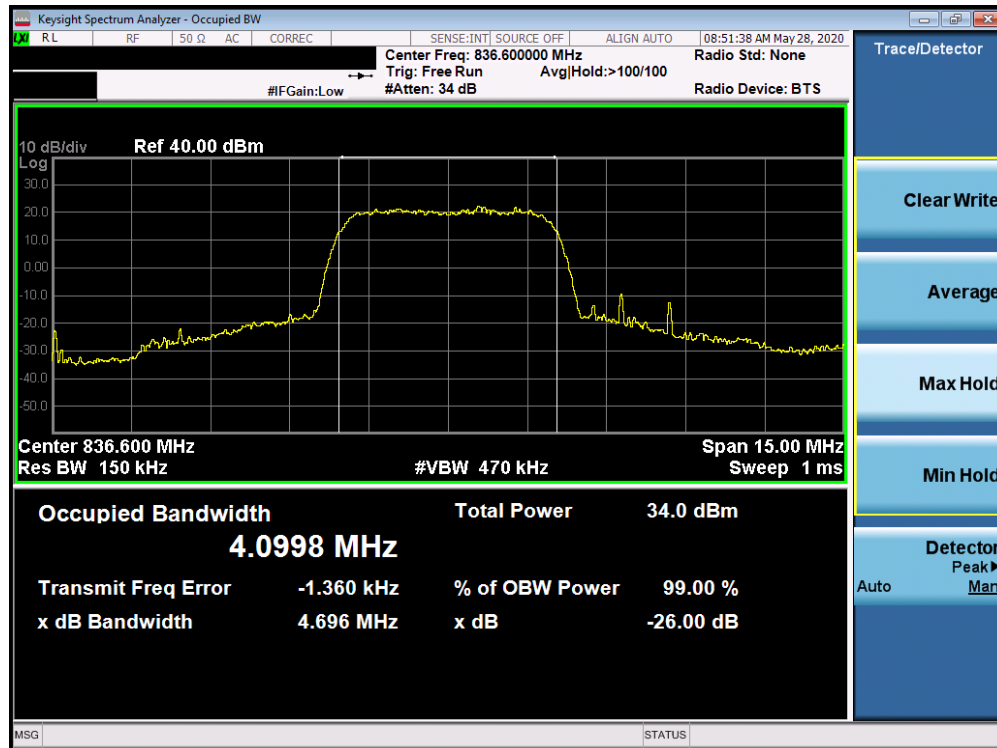
Plot 7-1. Occupied Bandwidth Plot (Cellular WCDMA Mode)
