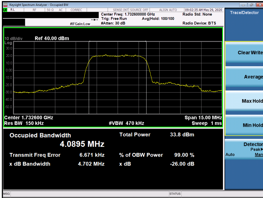
Plot 7-2. Occupied Bandwidth Plot (AWS WCDMA Mode)
