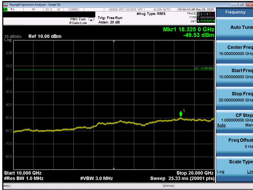
Plot 7-21. Conducted Spurious Plot (AWS WCDMA Mode - High Channel)
