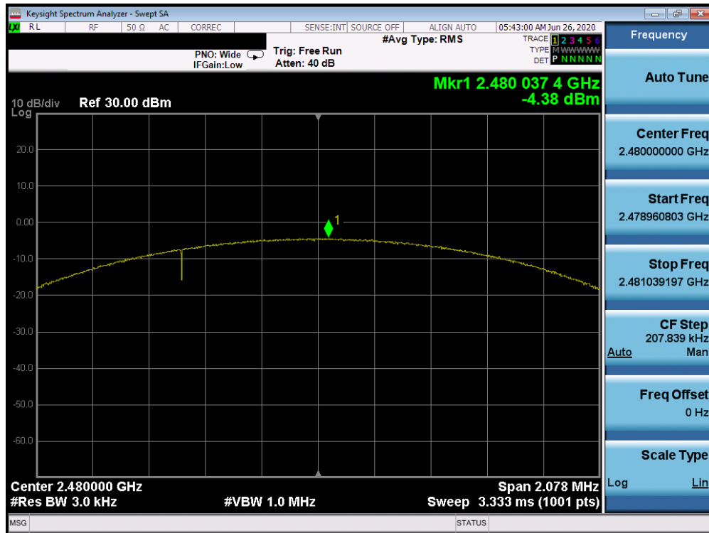
Plot 7-15. Power Spectral Density Plot (Bluetooth (LE), 2Mbps, ePA – Ch. 39)
