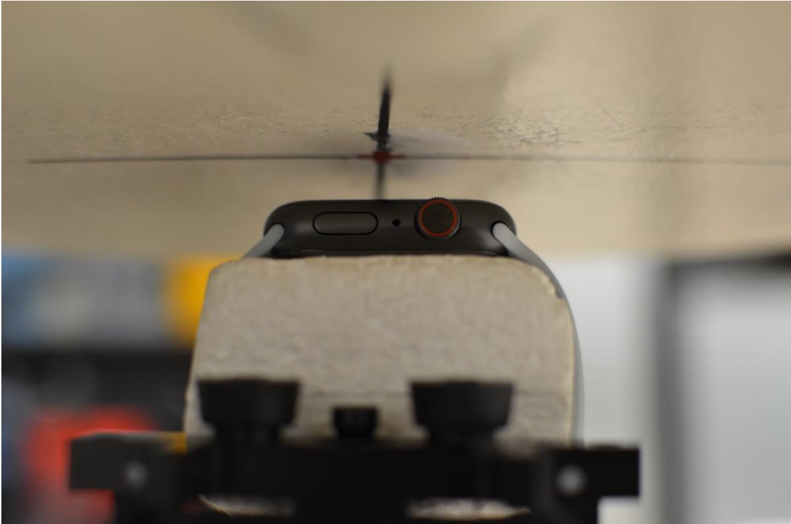
SAR Test Setup Photo 1: Aluminum with Sport Wristband, Front Side at 1.0 cm
