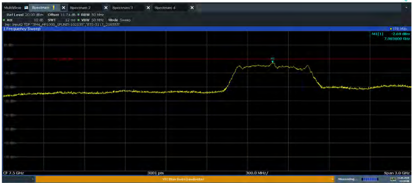
Plot 7-56. Peak Radiated Power (Ch. 9, Config 1/Payload 125)
