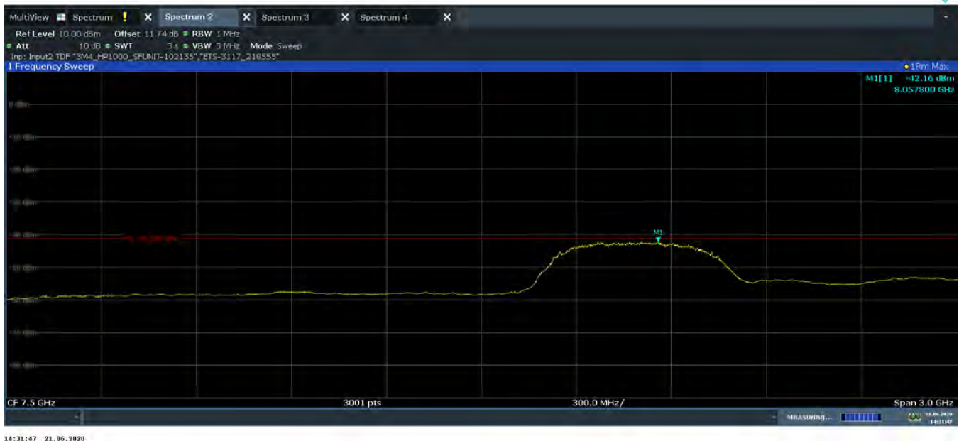
Plot 7-79. Average Radiated Power (Ch. 9, Config 4/Payload 0)
