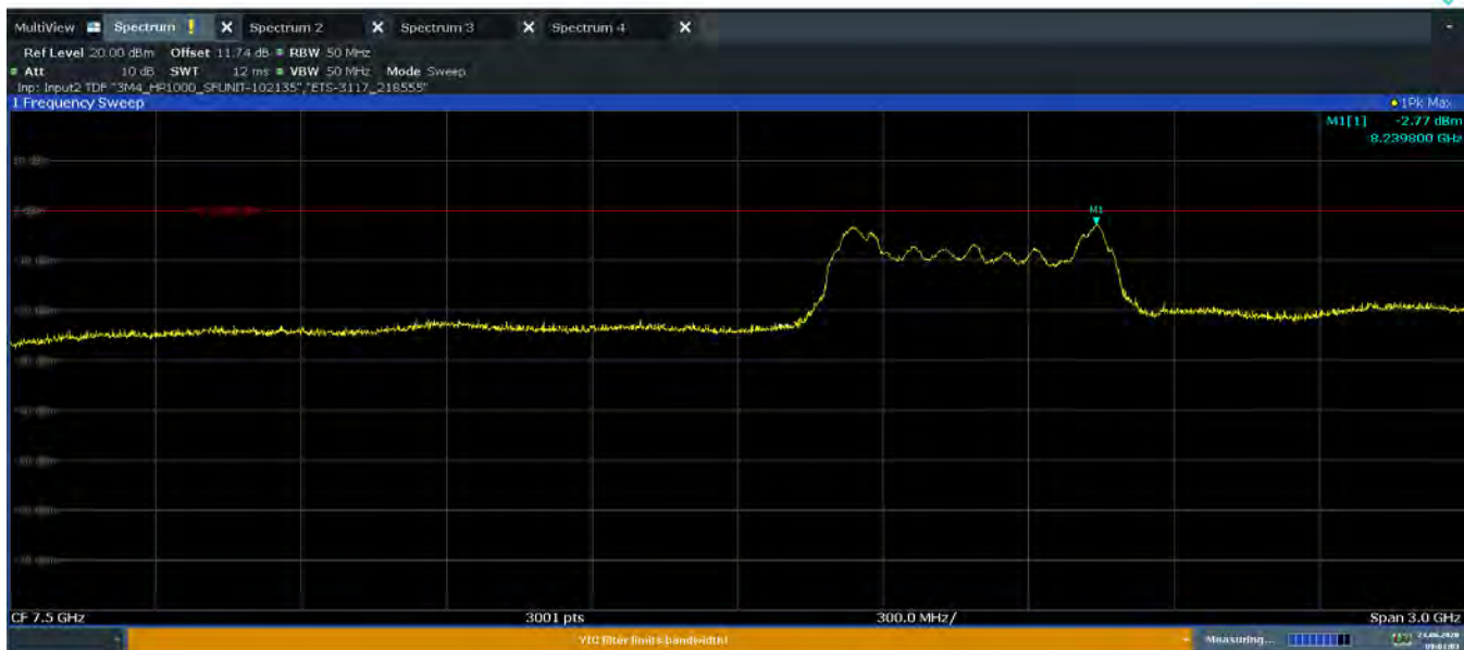
Plot 7-60. Peak Radiated Power (Ch. 9, Config 5/Payload 0)
