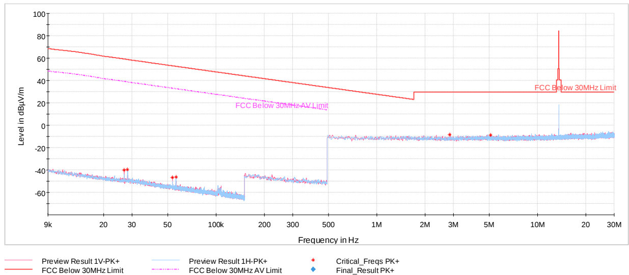
Plot 7-8. Radiated Spurious Emissions 9kHz – 30MHz (CE A 848kbps, with WCP + AC/DC Adapter)
