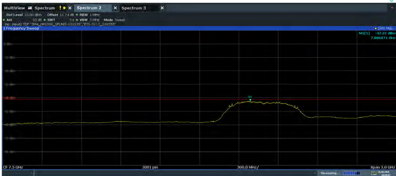
Plot 7-74. Average Radiated Power (Ch. 9, Config 1/Payload 45)
