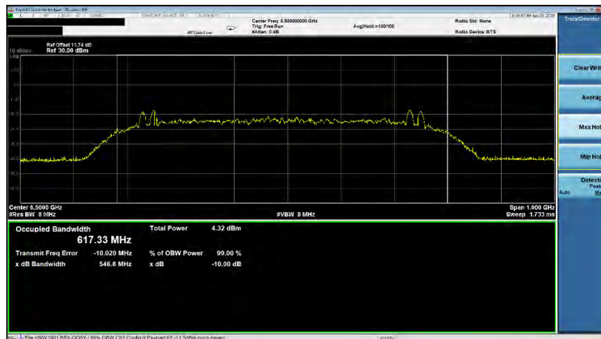
Plot 7-23. ISSED Occupied Bandwidth (Ch. 5, Config 0/Payload 125)
