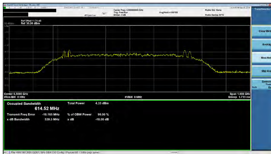
Plot 7-26. ISED Occupied Bandwidth (Ch. 5, Config 1/Payload 125)
