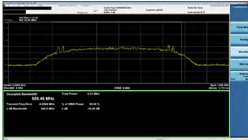
Plot 7-32. ISD Occupied Bandwidth (Ch. 9, Config 0/Payload 65)
