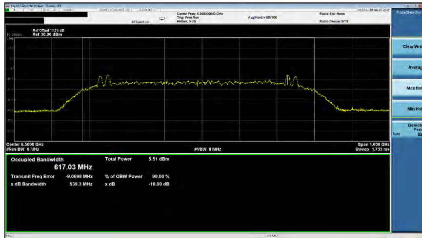
Plot 7-21. ISSED Occupied Bandwidth (Ch. 5, Config 0/Payload 25)
