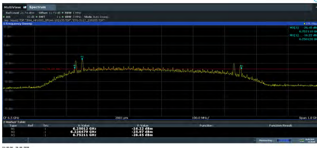
Plot 7-9. 10dBc Bandwidth (Ch. 5, Config 4/Payload 0)
