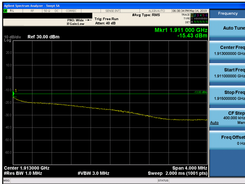
Plot 7-40. 4MHz Span Plot (PCS WCDMA Mode - High Channel)
