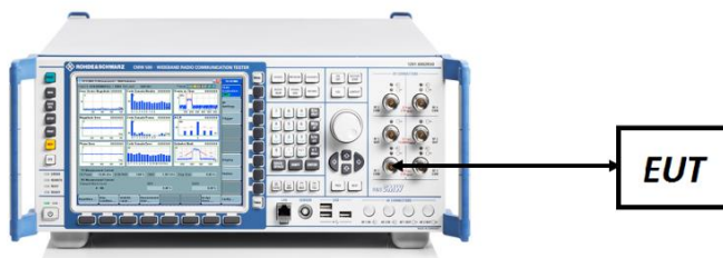
Figure 7-5. ERP/EIRP Measurement Setup
