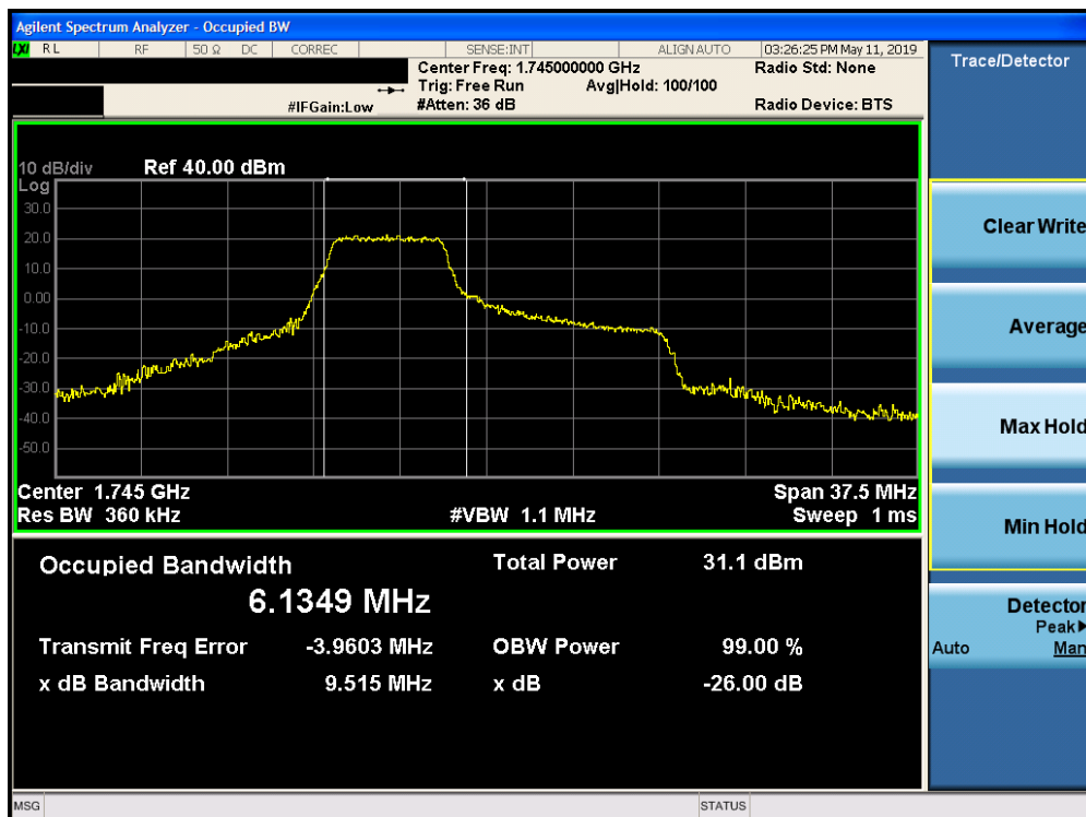
Plot 7-18. Occupied Bandwidth Plot (Band 66/4 - 15.0MHz 16-QAM - Full RB (27/0) Configuration)
