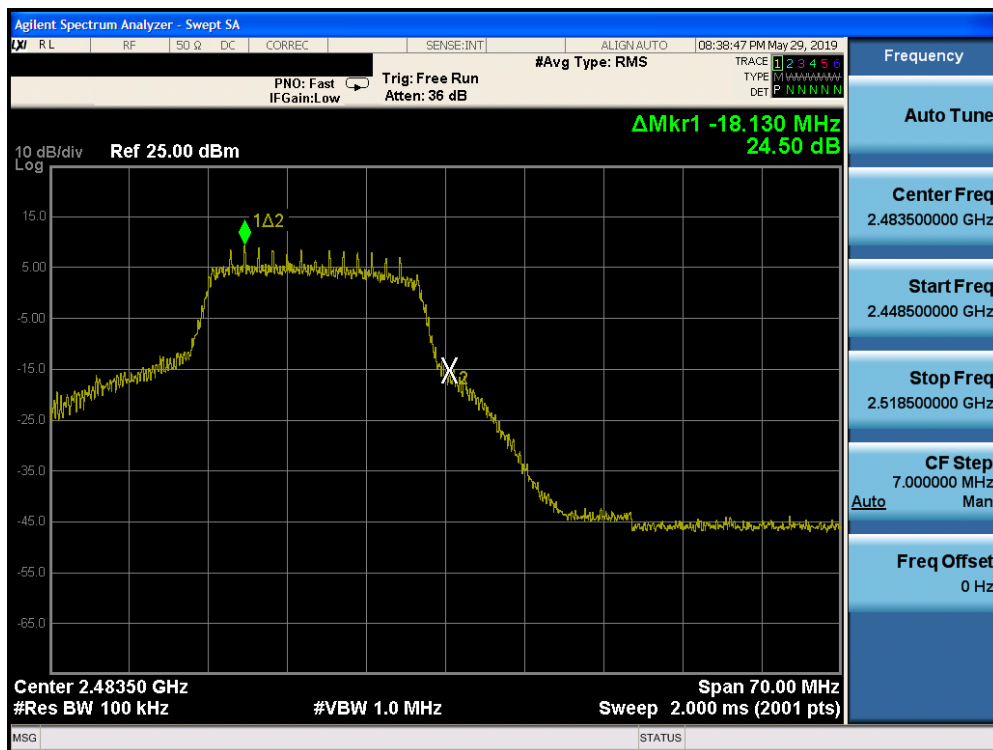
Plot 7-30. Band Edge Plot (802.11n (2.4GHz) – Ch. 13)
