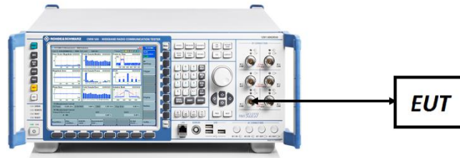
Figure 7-4. Conducted Power Measurement Setup
