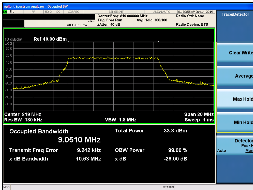
Plot 7-7. Occupied Bandwidth Plot (LTE Band 26, 10MHz QPSK – RB Size 50)
