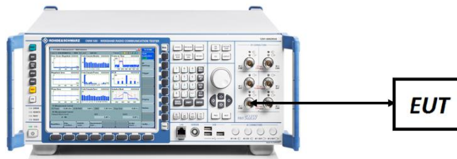
Figure 7-5. ERP/EIRP Measurement Setup
