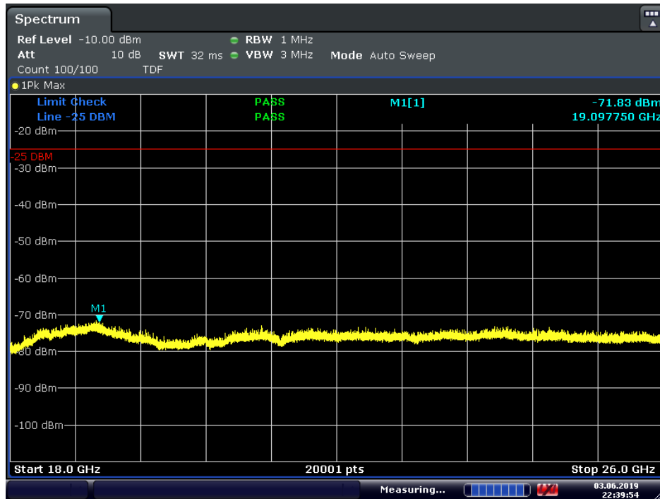
Plot 7-323. Radiated Spurious Plot 18GHz – 26GHz (Band 7, Pol. H)
