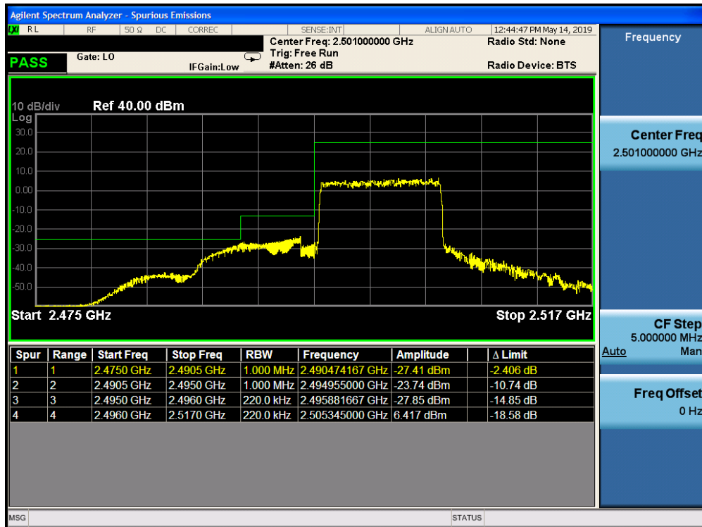
Plot 7-262. Lower ACP Plot (Band 41 - 10.0MHz QPSK - Full RB Configuration)
