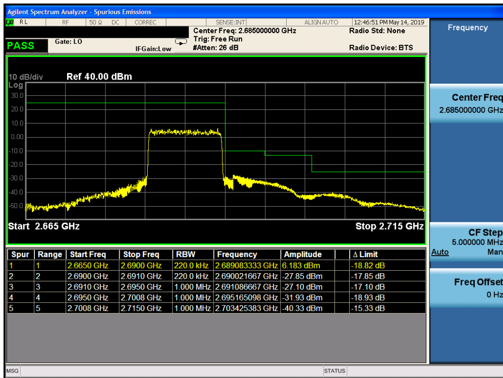
Plot 7-263. Upper ACP Plot (Band 41 - 10.0MHz QPSK - Full RB Configuration)
