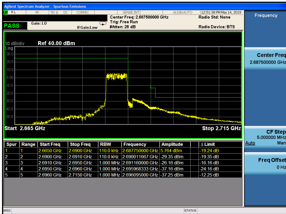
Plot 7-261. Upper ACP Plot (Band 41 - 5.0MHz QPSK - Full RB Configuration)
