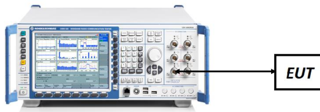
Figure 7-5. ERP/EIRP Measurement Setup
