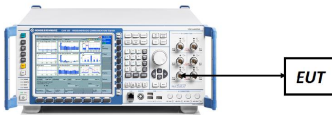
Figure 7-5. ERP/EIRP Measurement Setup
