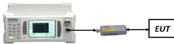
Figure 7-2. Test Instrument & Measurement Setup for Average Power Measurement
