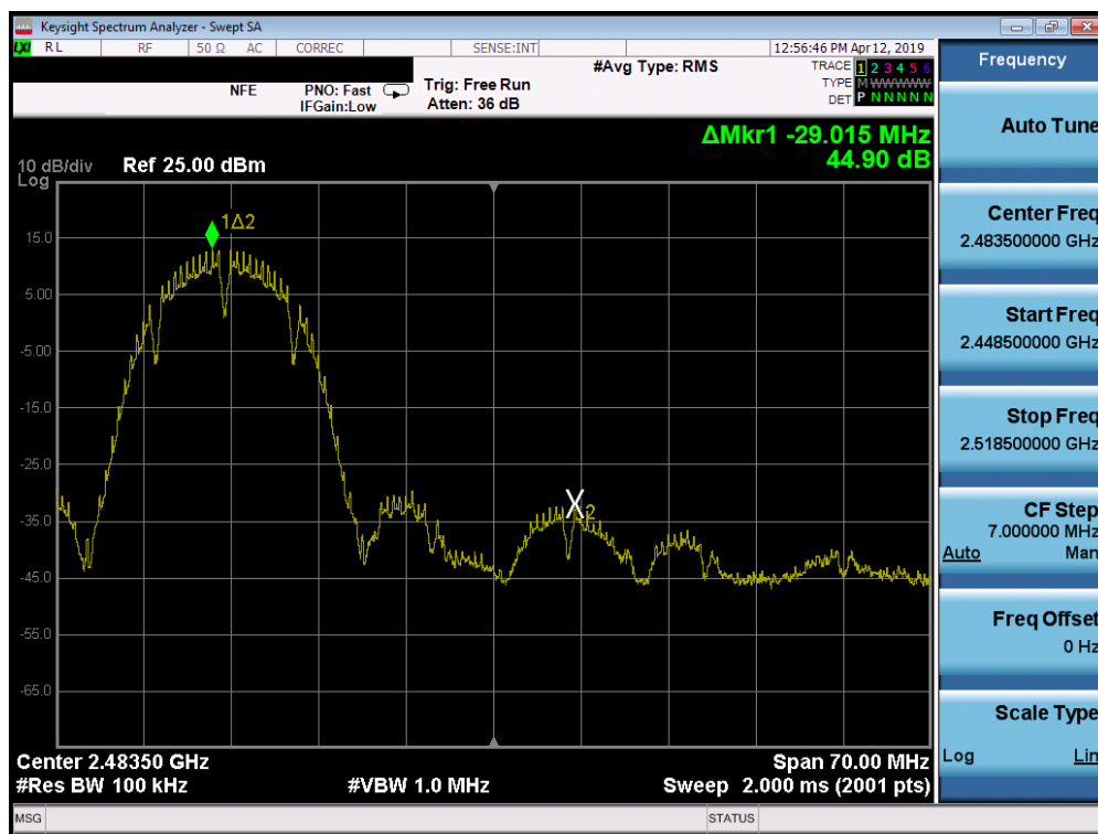
Plot 7-20. Band Edge Plot (802.11b – Ch. 11)
