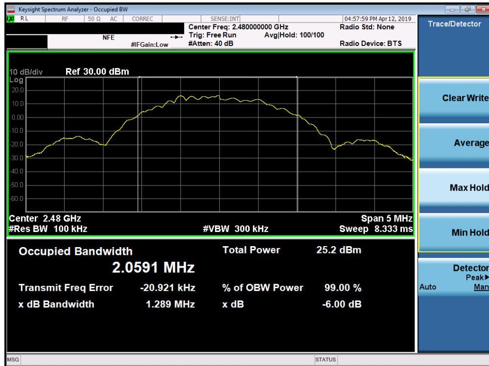
Plot 7-6. 6dB Bandwidth Plot (Bluetooth (LE), ePA – Ch. 39)
