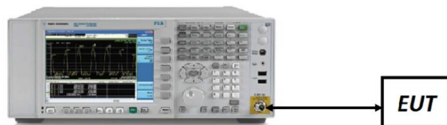
Figure 7-3. Test Instrument & Measurement Setup
