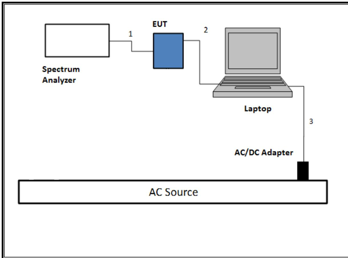
**SETUP DIAGRAM FOR RADIATED TESTS ABOVE 1GHz**
