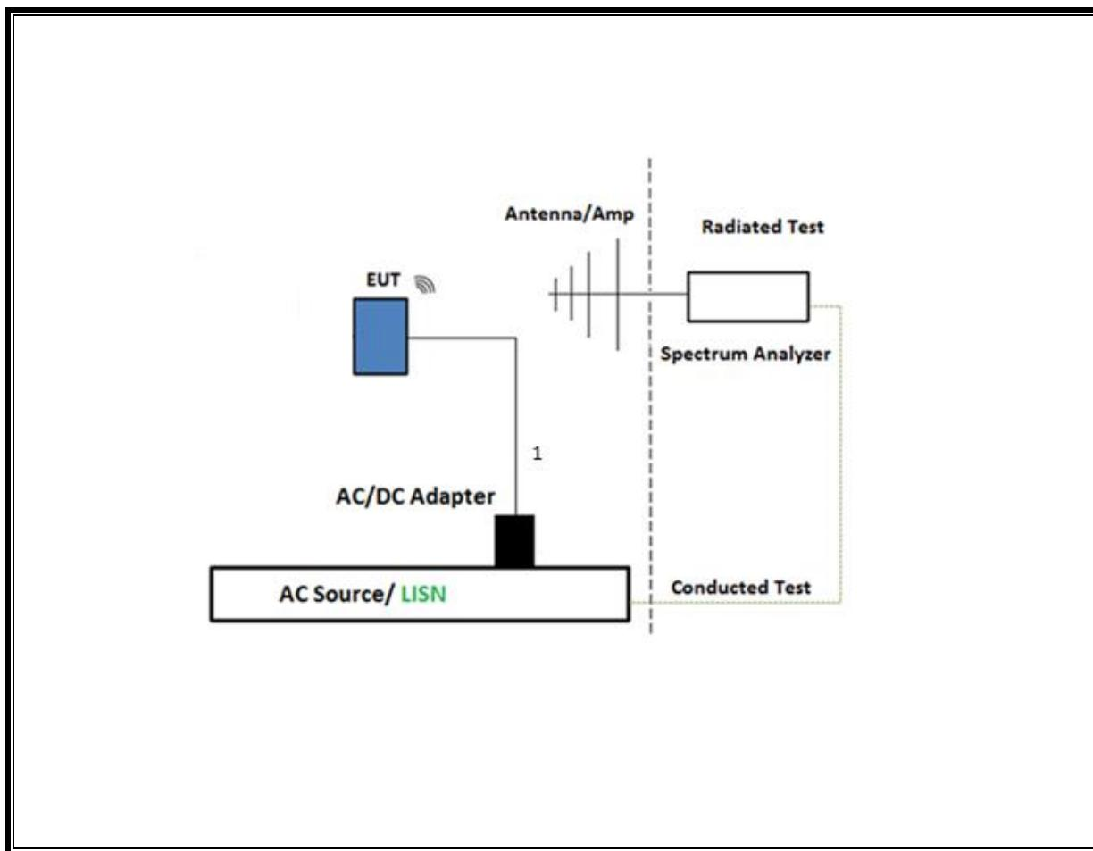
**TEST SETUP- AC LINE CONDUCTED: LAPTOP CONFIGURATION**
