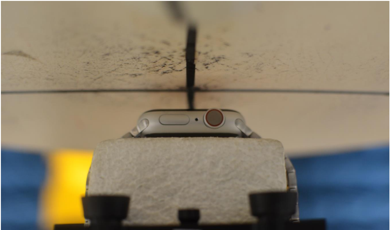
SAR Test Setup Photo 2: Aluminum with Metal Links wristband, Front side at 1.0 cm
