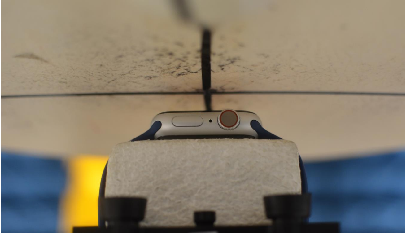
SAR Test Setup Photo 1: Aluminum with Sport wristband, Front side at 1.0 cm
