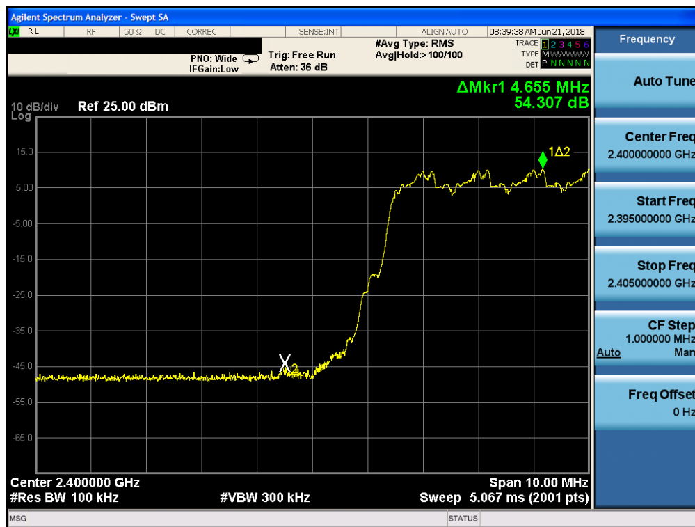
Plot 7-39. Band Edge Plot (Bluetooth with Hopping Enabled, 8DPSK, iPA)
