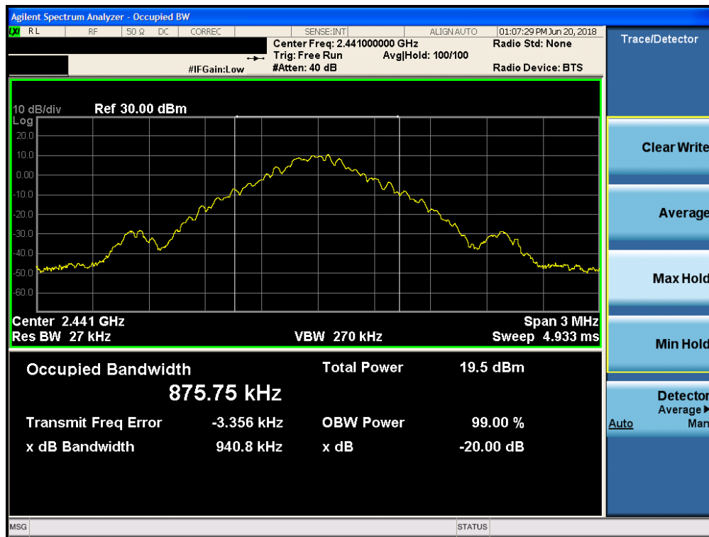
Plot 7-5. 20dB Bandwidth Plot (Bluetooth, GFSK, iPA – Ch. 39)
