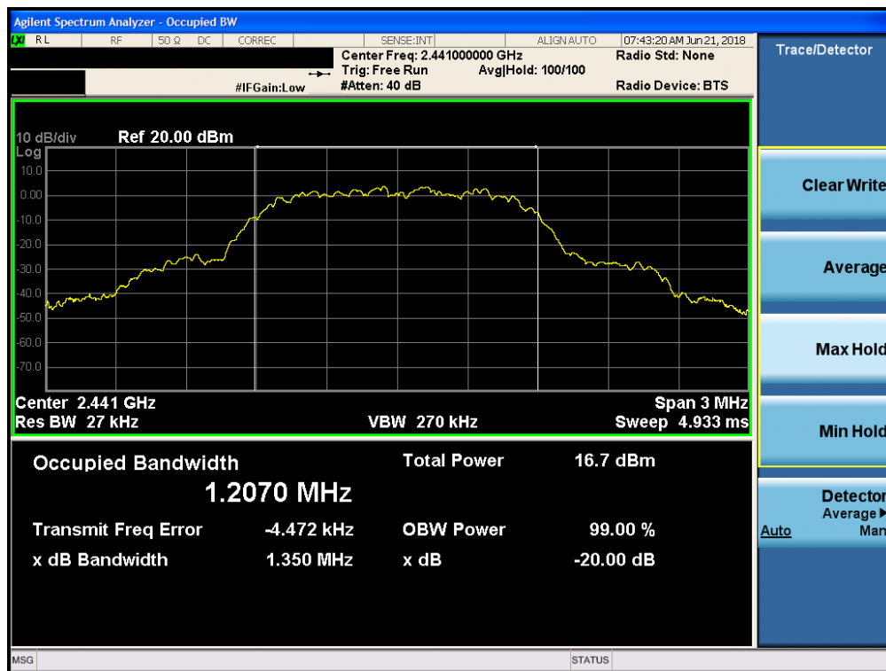
Plot 7-11. 20dB Bandwidth Plot (Bluetooth, 8DPSK, iPA – Ch. 39)
