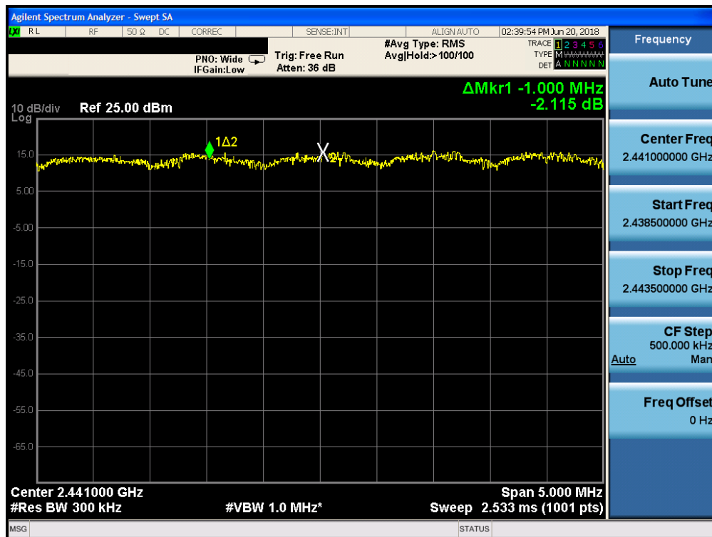
Plot 7-42. Channel Spacing Plot (Bluetooth, 8DPSK, ePA)
