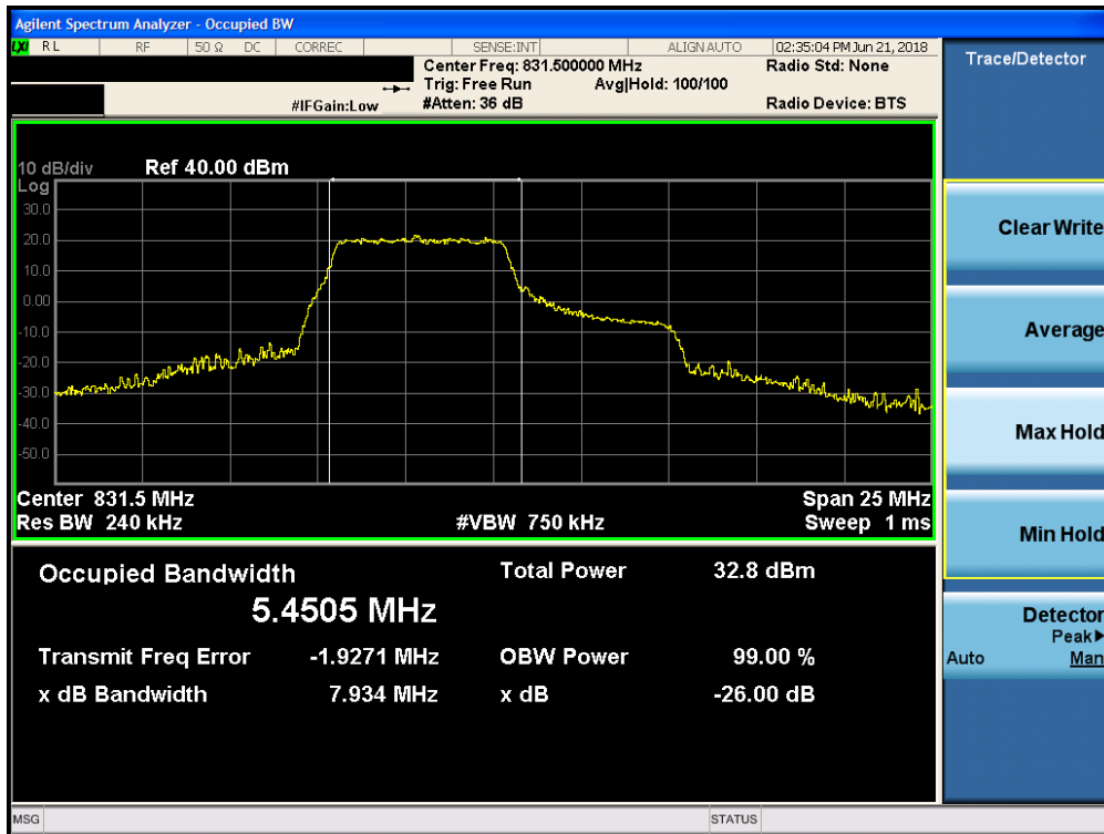
Plot 7-8. Occupied Bandwidth Plot (Band 26/5 - 10.0MHz 16-QAM - RB Size 27, RB Offset 0 Configuration)
