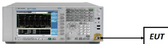
Figure 7-7. Test Instrument & Measurement Setup
