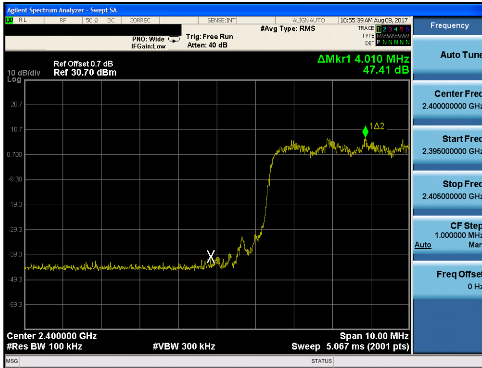
Plot 7-19. Band Edge Plot (Bluetooth with Hopping Enabled, \pi/4 DQPSK – Ch. 0)
