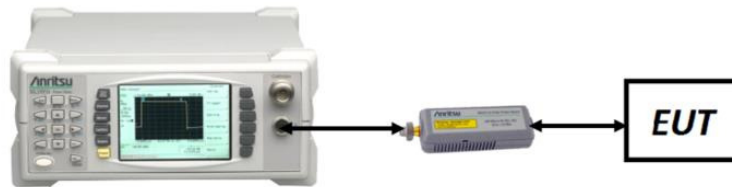
Figure 7-3. Test Instrument & Measurement Setup for Average Power Measurement
