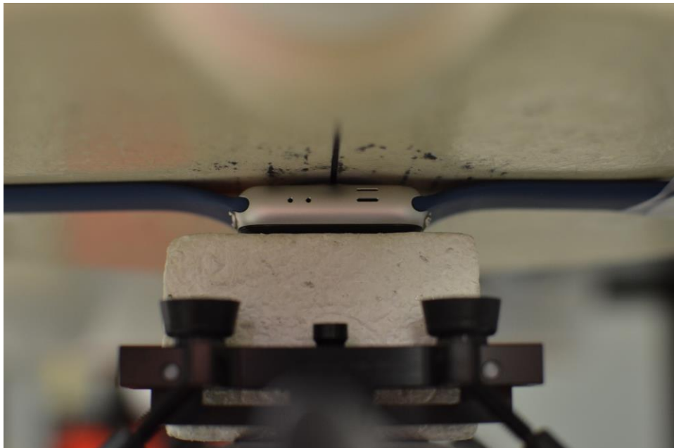
SAR Test Setup Photo 12: Aluminum with Sport wrist band, Back side at 0.0 cm
