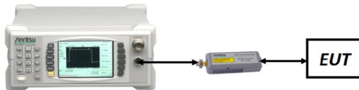
Figure 7-3. Test Instrument & Measurement Setup for Average Power Measurement
