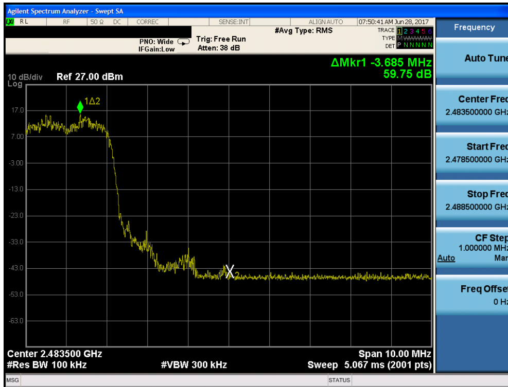
Plot 7-36. Band Edge Plot (Bluetooth with Hopping Enabled, 8DPSK, ePA - Ch.78)
